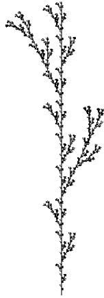
Figure 5.8: This tree is generated using the following L-System: \omega : F , R : F- \rightarrow F[+F]F[-F]F . \delta is 25 degrees and this is the fifth iteration.
