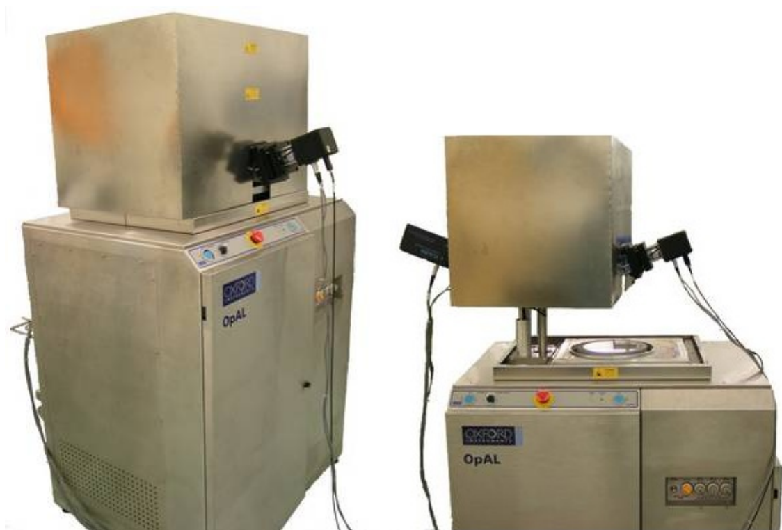
Figure 19: The atomic layer deposition machine used in the growth of our samples. The spectroscopic ellipsometry viewports are clearly visible. [23]
