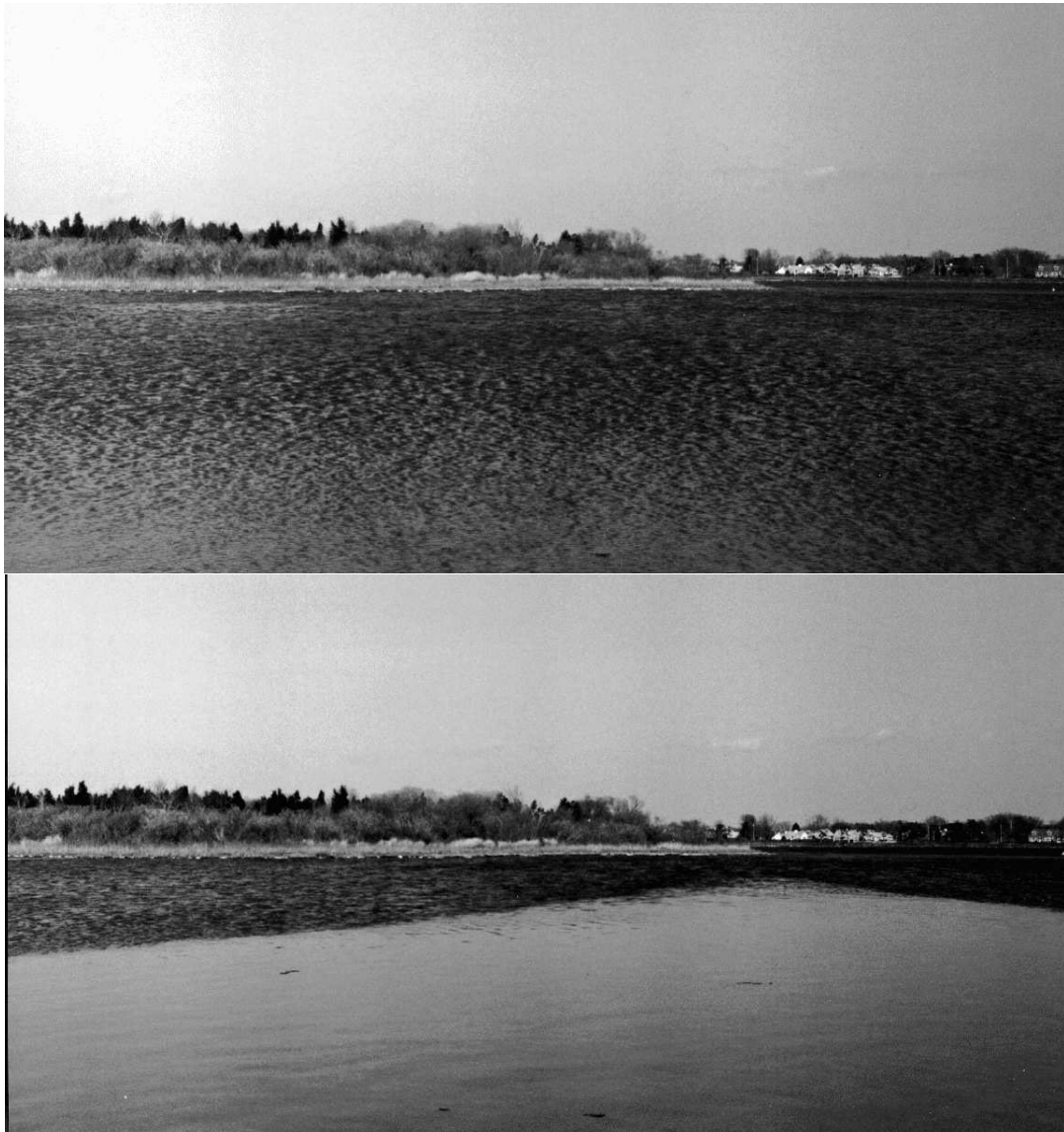
Figure 1.1: Recreated Franklin experiment. The upper photo shows the water condition prior to the addition of oil. The lower picture shows the condition after the addition of oil [15]
