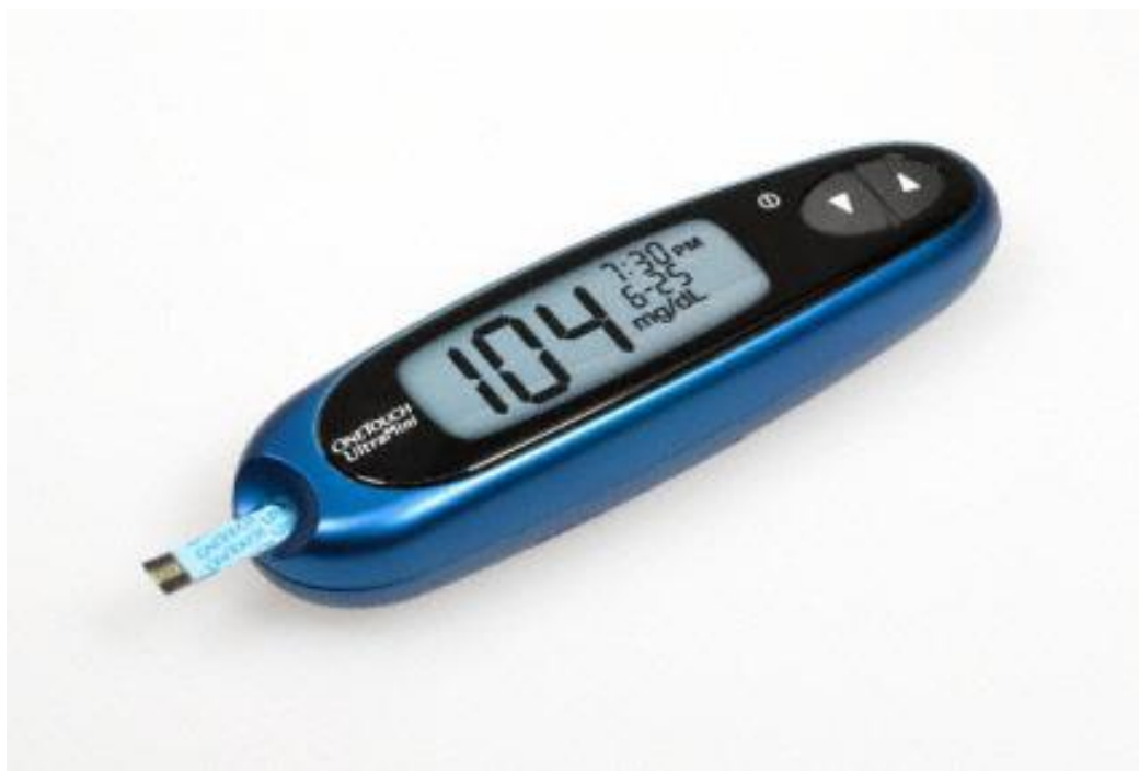
Figure 1: A blood glucose meter (OneTouch® UltraMini®), is a common example of a biosensor [3].
