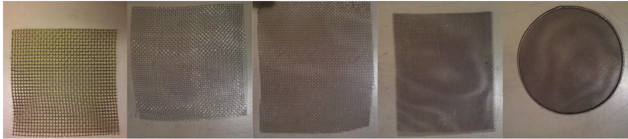
Figure 6: Used meshes of different gap widths and wire thicknesses. From left to right will be numbered mesh 1 to mesh 5
