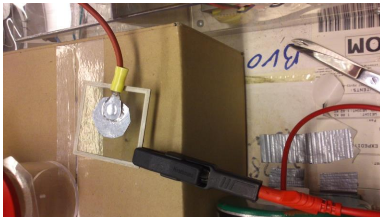
Figure 9: Connecting the ITO to the main setup using aluminum tape.
