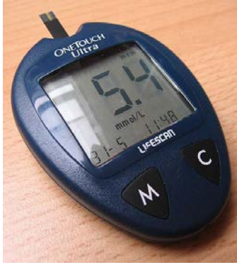
Figure 1a (left): A modern day glucose biosensor. Figure 1b (right): The schematic reaction chain in which a single glucose molecule is detected. Under influence of glucose oxidase, glucose is oxidized, forming hydrogen peroxide and GDL. The H_2O_2 then takes part in a redox reaction with horseradish peroxidase (HRP) as catalyst, using one electron, forming a current when more glucose molecules are present in the sample.
