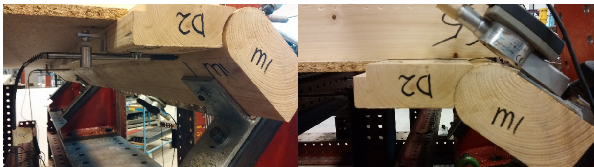
Figure 4.3d; Pictures of the wall plate M1 and supporting batten D2 and the existing gap on the left before testing, and the non-existing gap on the right once 2kN of horizontal axial force is applied
