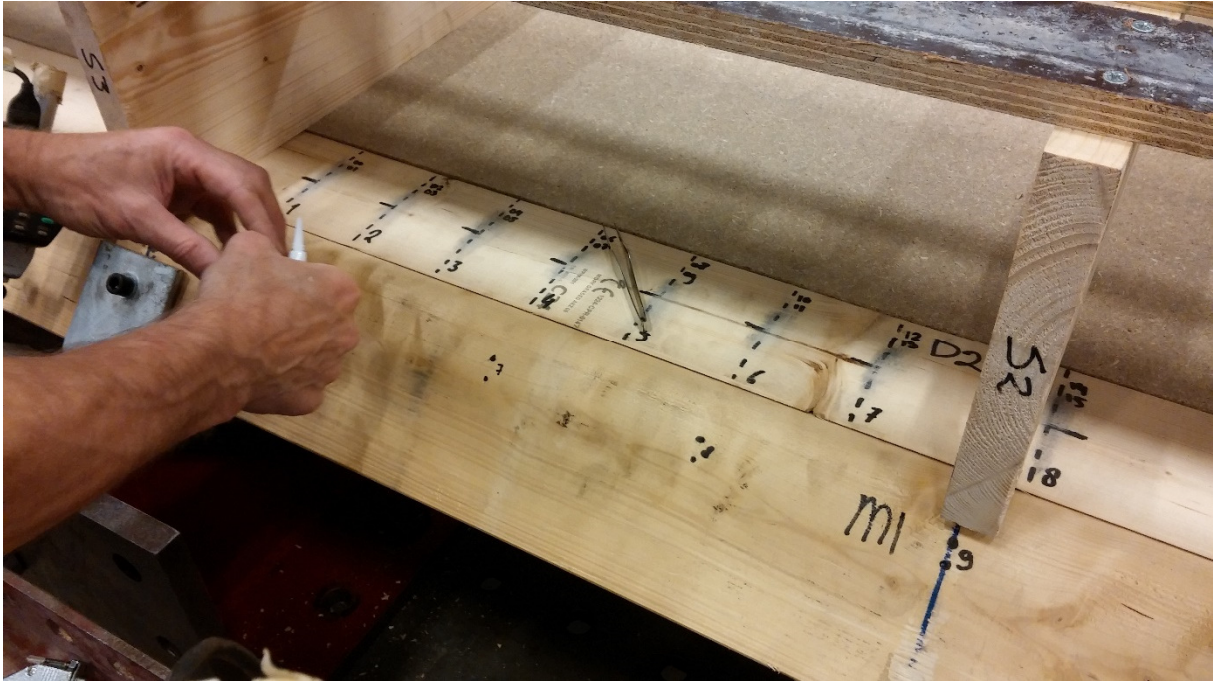
Figure 4.4o; Positions of the strain gauges on the supporting batten. On the right side the dislocated position 8 giving abnormal results
