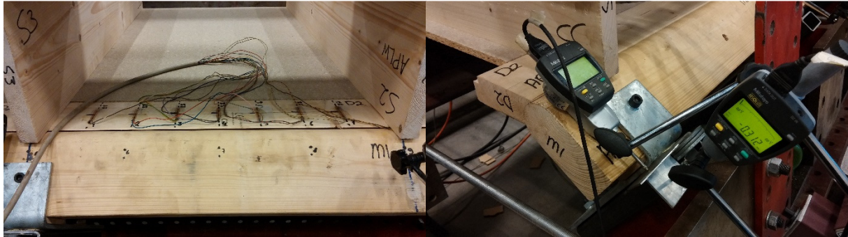
Figure 4.3N; Left: Strain gauges attached to the upper side of the supporting batten Right: LVDT's measuring the set-up for abnormal behavior
