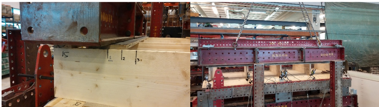
Figure 4.3M; Left: Specified position for the dead load which leads to about 10% of load loss Right: The dead load is applied with the use of a crane
