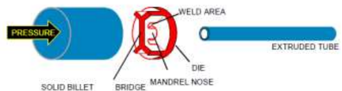
Figure 3.6. Extrusion of hollow section (TALAT 1302, 1994)
