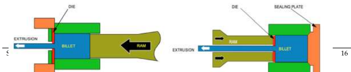
Figure 3.4. Direct (left) and indirect (right) extrusion process (TALAT 1302, 1994)
