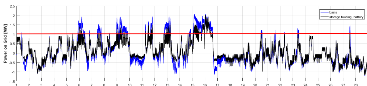
Figure 14 - Power fluctuation on grid connection for February with storage in the building and battery
