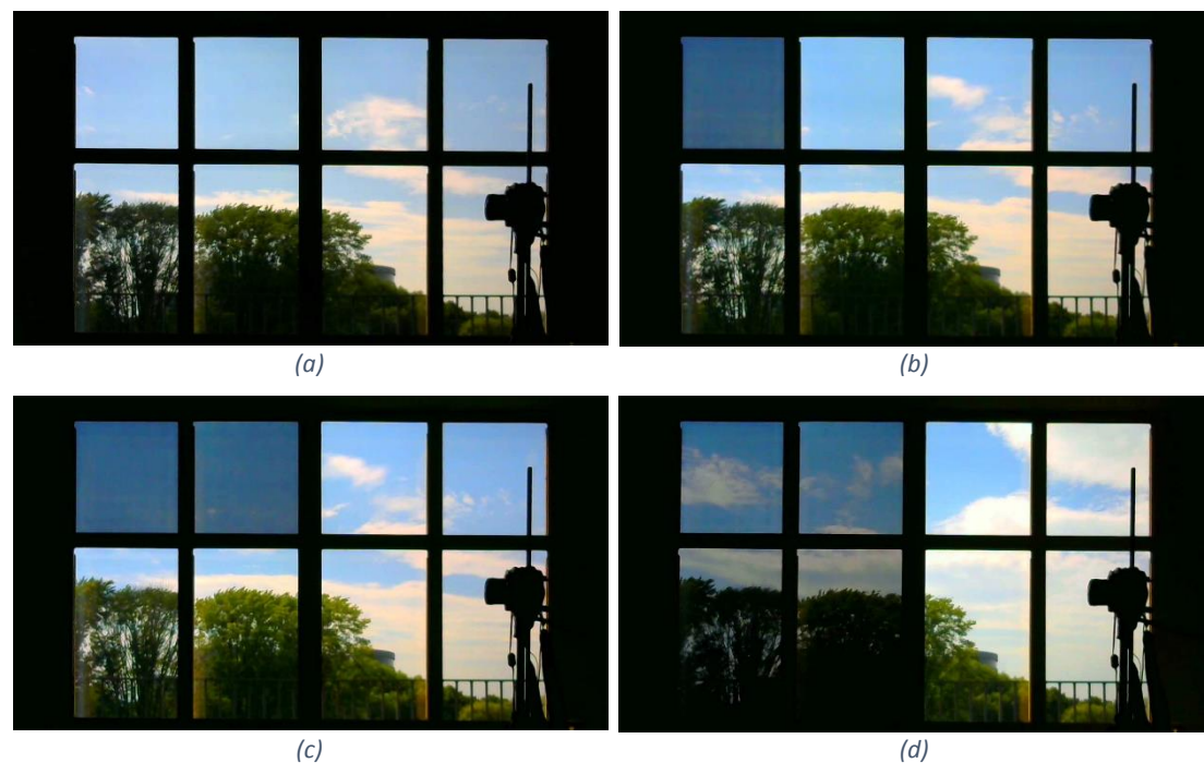
Figure III-24: (a-b-c-d) Operation sequence of GPC control strategy in the pilot study, from 14:00 to 17:00 on Friday 5 th of August 2016.
