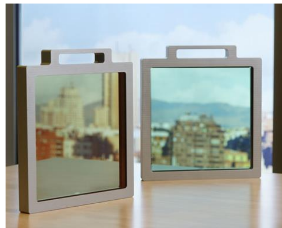
Figure I-4: (a) DDLC technical specifications. (b) The appearance of the glazing system in the dark and bright state, respectively on the left and on the right.
