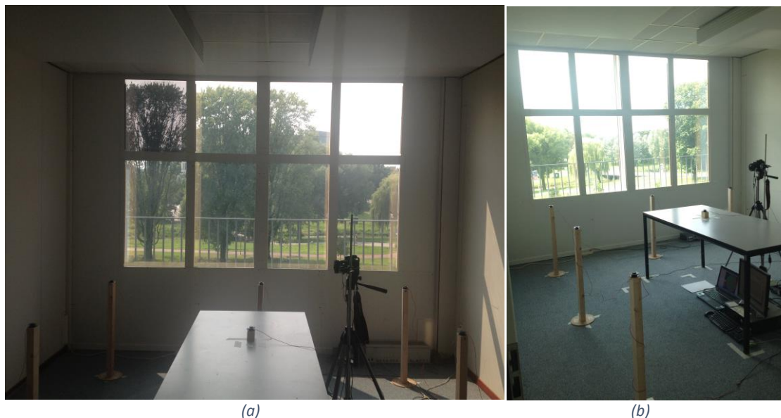
Figure III-21: (a)(b) Final set-up of the pilot study implementing: the DDLC façade array controlled by GPC control strategy 'Pixel', the workstation, the view point (i.e. luminance camera and sensor), and the grid of sensors. (b) The laptop enabling the control system is placed under the desk to avoid disturbances to the measurements.
