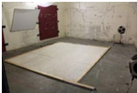
Figure 6.10: WWCBs in the reverberation room of Peutz in Mook, the Netherlands.
