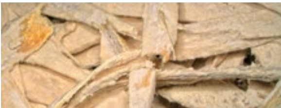
Figure 5.7: Microscopic picture of a WWCB using a Microscopic Keyence: Damage of the wood fibres during the production process.
