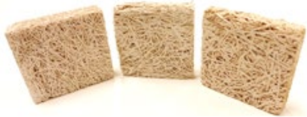
Figure 5.1: From left to right: WWCB-samples with 1.0, 1.5 and 2.0 mm fibres.
