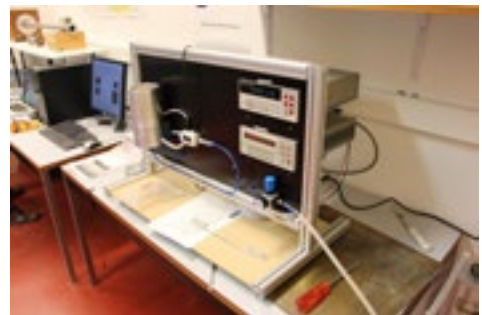
Figure 5.12: Schematic overview (left) and a picture (right) of the flow resistivity measurements.
