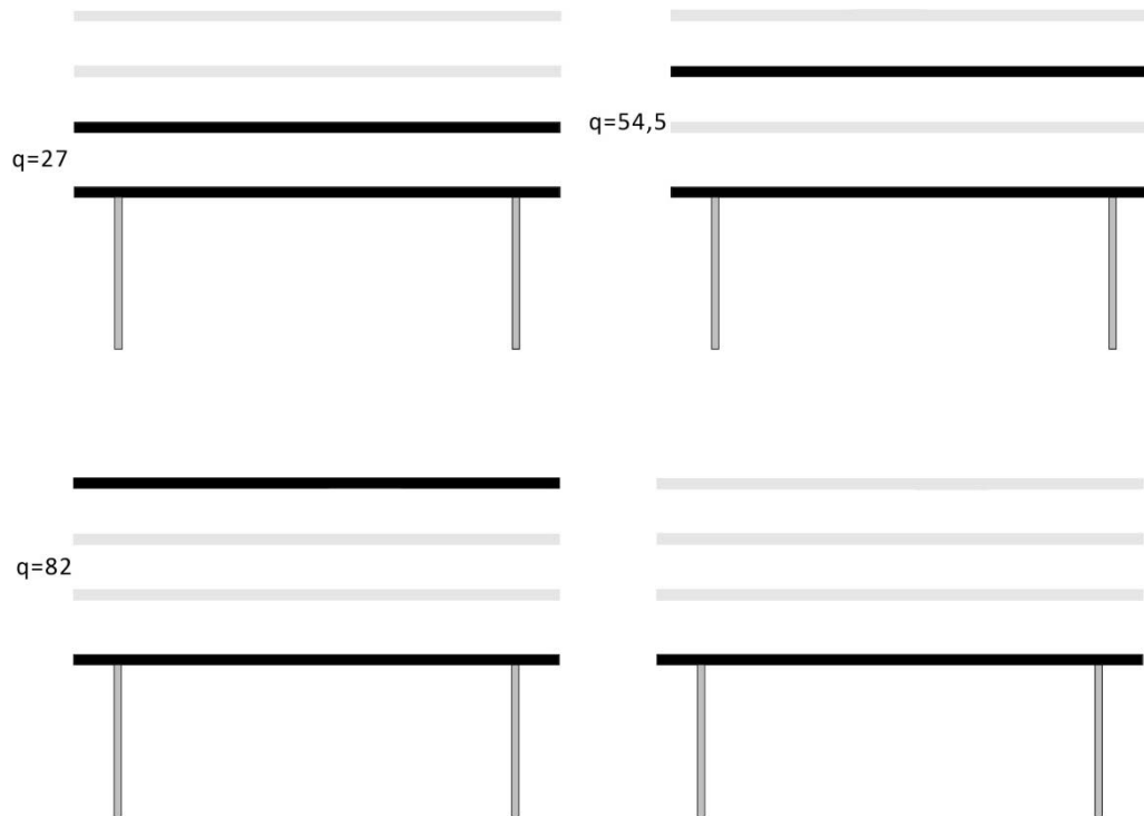
Figure 5.6 Different measurement situations with height of the panel above the table q (cm)
