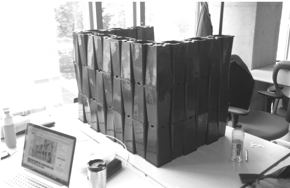
Fig. 46 – Small scale test with flower pot stacked to form walls
