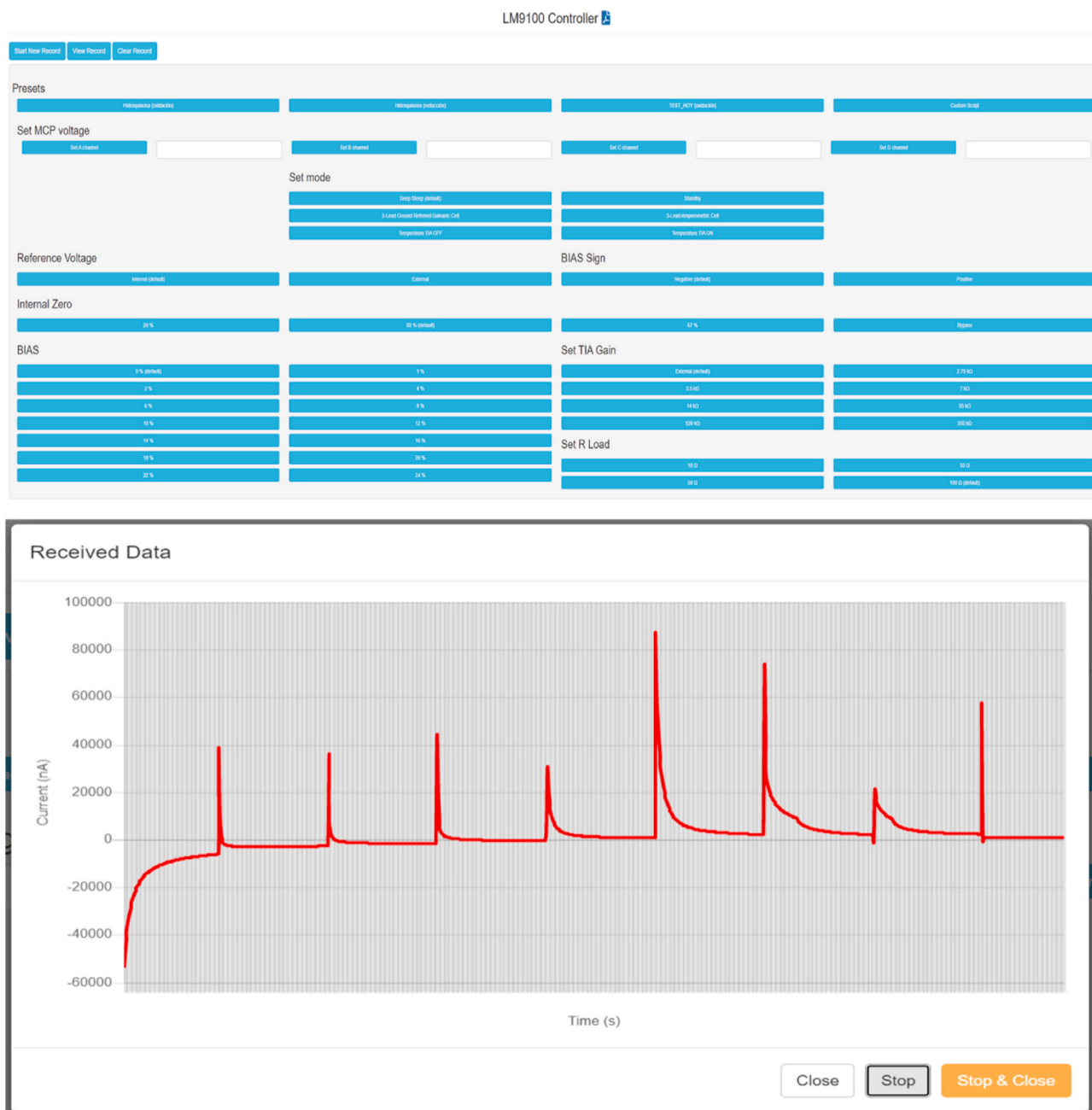
Fig. 3. Web Interface and an example of Data Sample Graph.
