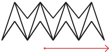
Concept 3: A serie of connected triangles that can be unfolded into trusses
