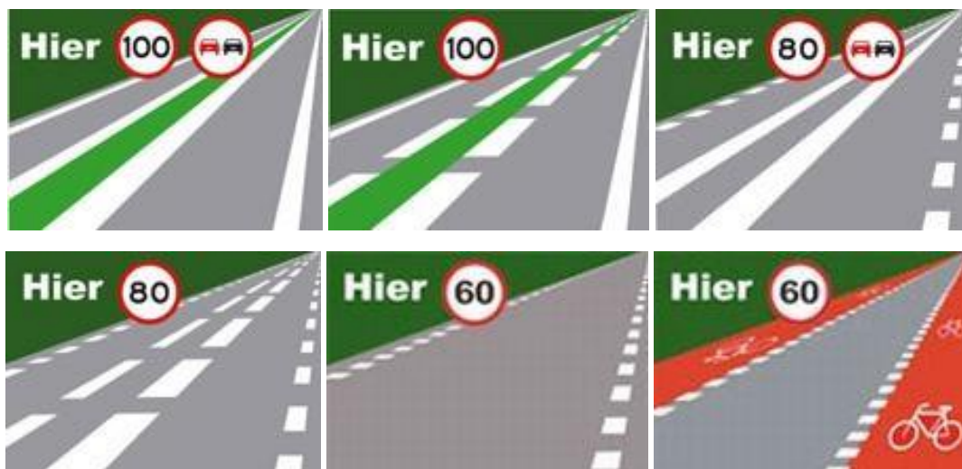
Figure 4: Design of road markings with their matching speed limit for different road types. Verkeer - Nederlandse wegen - Belijning en maximumsnelheid, 2008.
