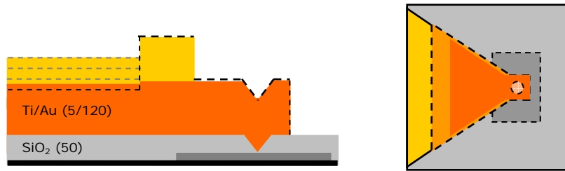
Figure 4-3-I: The tips in the cured FOX12 are transferred to the uniform Au layer by ion-milling. At the same time, the top electrodes already in place get milled as well. Inserting an additional hard buffer layer on top of the electrodes can provide thicker electrode thicknesses, as indicated by the dashed lines. The maximum thickness of the tip is obtained by stopping the ion-milling exactly when the SiO 2 layer underneath has been reached. Over-milling results in thin tips that are subject to easy destruction by high currents.
