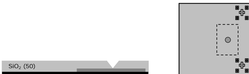
Figure 4-3-C: The nanometer scale point contact is defined with e-beam lithography in a single PMMA resist layer and etched into the underlying SiO 2 layer using a buffered hydrofluoric acid solution (BHF) that selectively etches SiO 2 . Etching stops on the underlying spin valve Pt capping layer.
