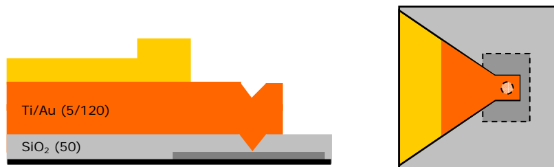
Figure 4-3-I: The final structure in side and top view. The small tips make contact with an extended magnetic layer through a nanometer scale point contact hole in the insulating SiO 2 layer. The current is effectively confined to a small area while the surrounding magnetic layer is accessible for optical measurements.
