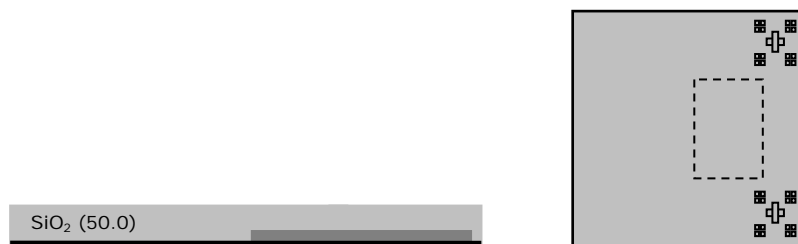
Figure 4-3-B: Passivation of the magnetic thin film elements. An intermediate Al(0.4) layer is deposited and plasma-oxidized, resulting in an Al 2 O 3 adhesion layer for the subsequently sputtered SiO 2 (50.0) layer.
