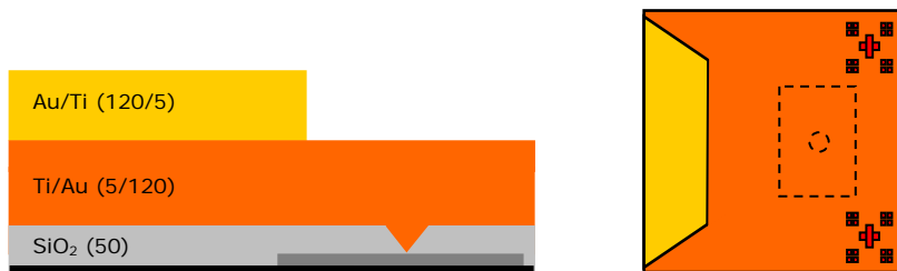
Figure 4-3-E: The main parts of the top electrodes are defined with optical lithography and lift-off of a sputtered Au(120.0)/Ti(5.0) layer. Only the small BLS tip ends on top of the point contacts remain to be defined in a later stage.
