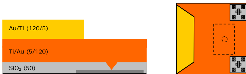
Figure 4-3-F: Before the small tips can be defined with e-beam lithography, the e-beam markers that were deposited in the first step (together with the rectangular magnetic thin film elements) have to be cleared using optical lithography and a chemical Au etch.
