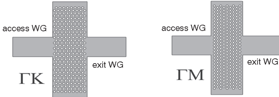
Figure 2.3: 2D hexagonal photonic crystals in \Gamma K and \Gamma M direction with access and exit waveguide (WG).
