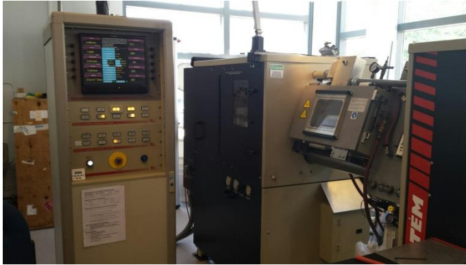
Figure 3.7 Test device Gleeble 3800
