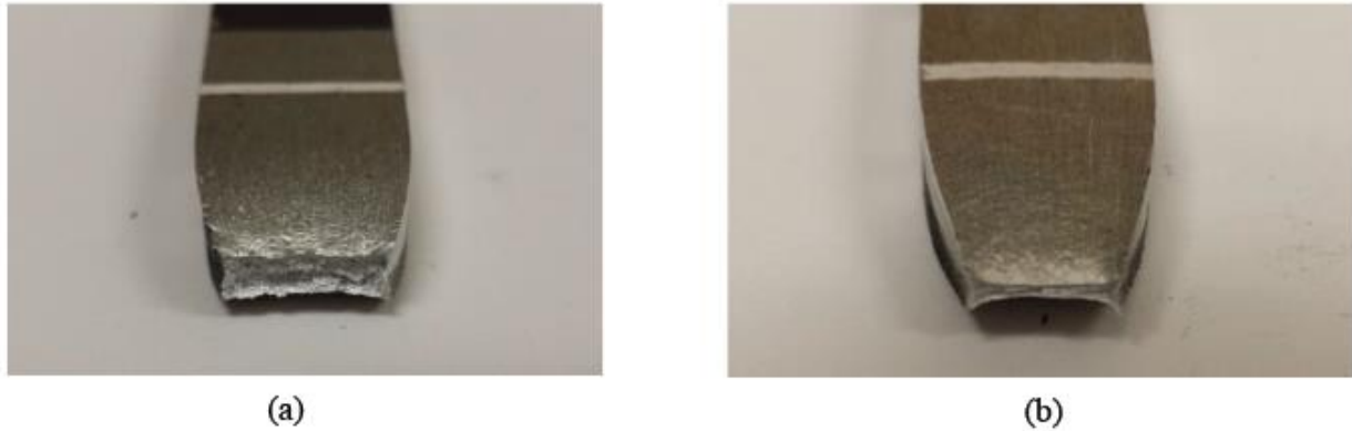
Figure 2.13 Fracture surface of thermo-mechanical tested samples (a) 300°C, (b) 400°C [Blakenship, 1996].
