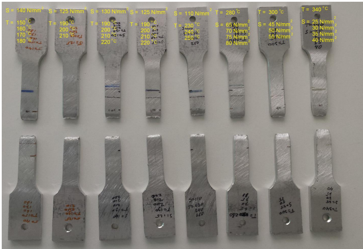
Figure 3.18 Reduction in area evolution of samples with a weld
