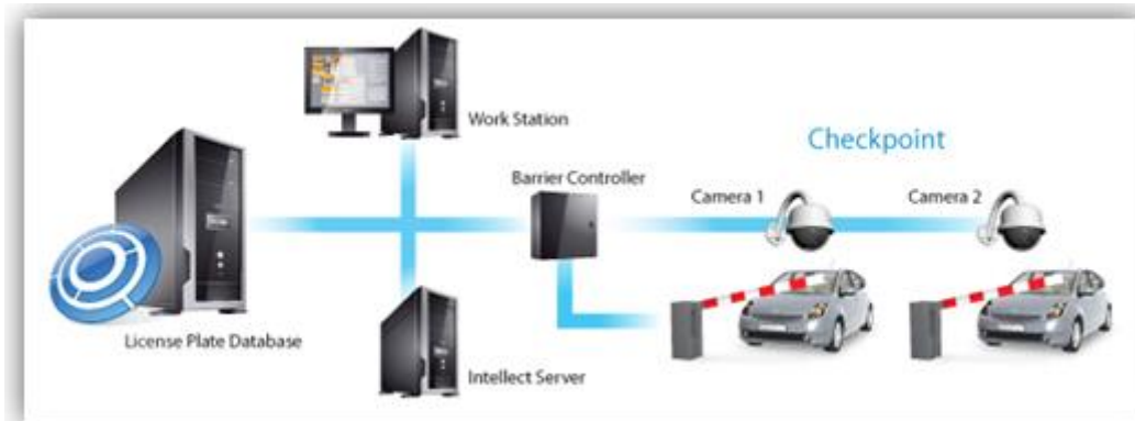
Figure 14 License Plate Recognition (FidPark, 2017)
