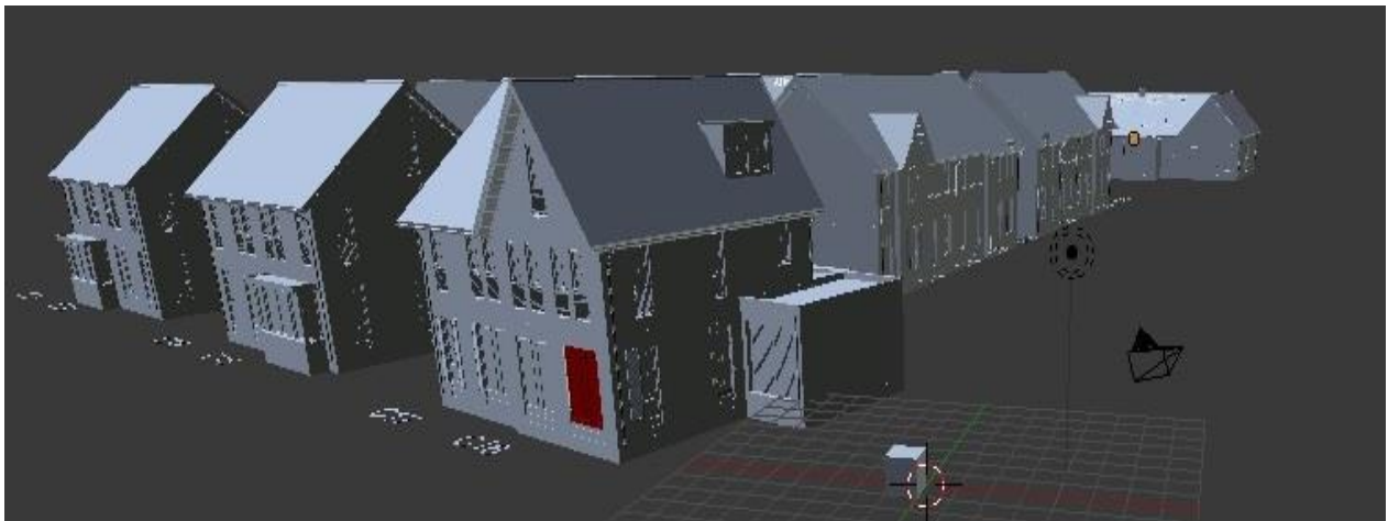
Figure 24: Color coded model – Rejected quality inspection example of a window
