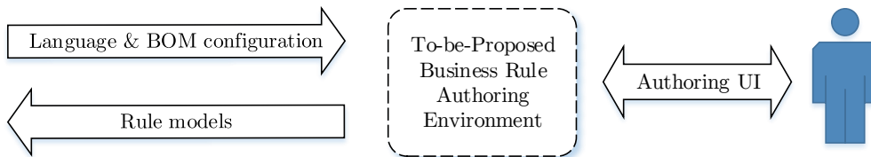
Figure 3.1: The dashed line denotes the boundary of the proposed system, the arrows denote the interfaces with surrounding systems.
