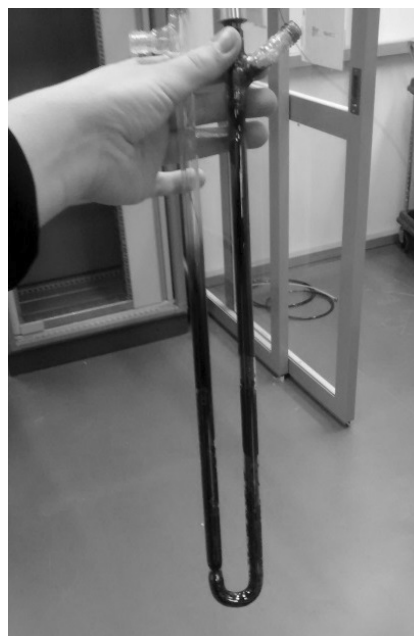
Fig. 62. Blackened reaction after toluene steam reforming reaction at 900 °C.
