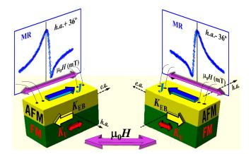
FIG. 1. Schematic representation of the chiral asymmetric transport behavior in FM/AFM system (as described in the text), which arises from interfacial exchange coupling. The intrinsic (two- fold)  $K_{\rm U}$  and interfacial-induced (one-fold)  $K_{\rm EB}$  anisotropies are indicated with arrows. The top graphs display the corresponding MR curves acquired around the h.a. direction.
