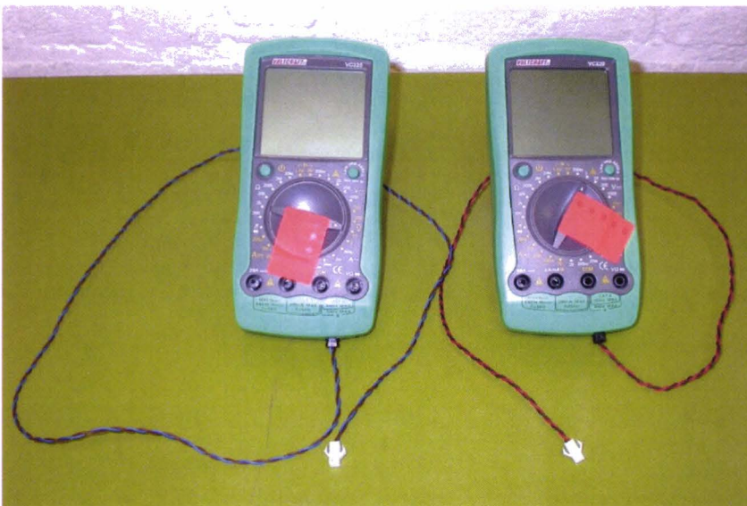
Figure 32. Modified multi meters for voltage measuring in assembly line
