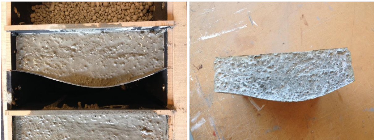
Figure 64a & Figure 64b: Concrete panel without any support
