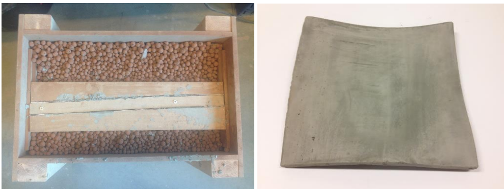
Figure 10a: The mould is fully poured with concrete & Figure 10b: The end result of a concrete casted panel
