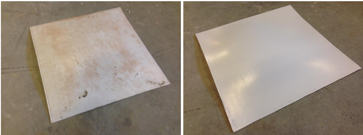
Figure 125a: The PS sheet after demoulding & Figure 125b: The PS sheet after cleaning
