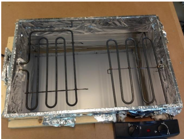
Figure 119a: The heating element consisting of two heating spirals & Figure 119b: Measurement temperature of the heating element
