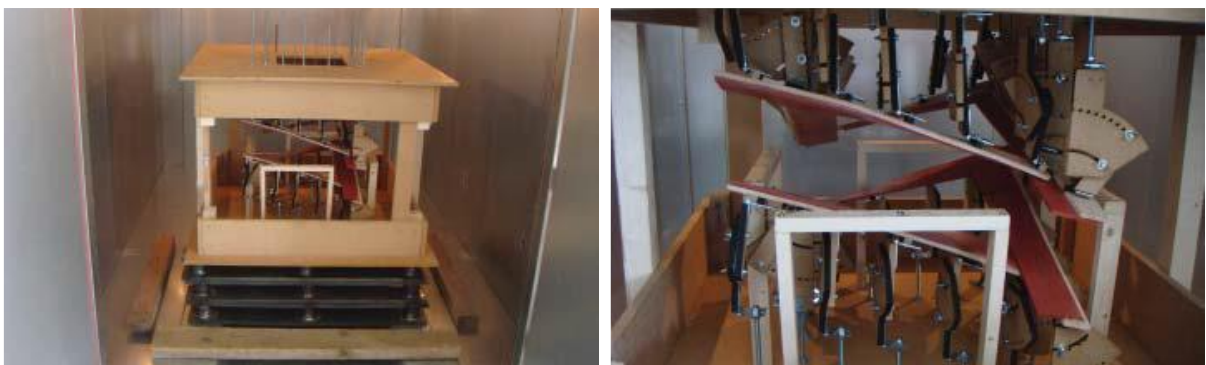
Figure 27a: Prototype of the Flexible Mould & Figure 27b: The actuators of the Flexible Mould (Gard, 2013)
