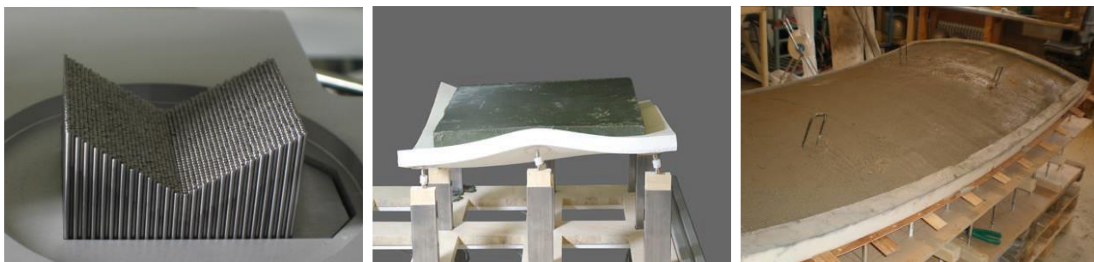
Figure 2a: Pinbed [3], Figure 2b: Zero-waste free-form formwork [4] & Figure 2c: Flexible mould [5]
