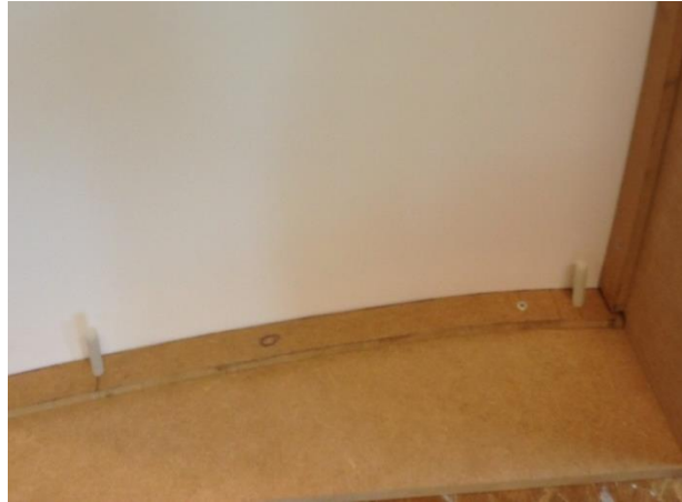
Figure 131a: Adjustable anchor (Fixinox, n.d.) & Figure 131b: Tubes fixated in mould for anchors
