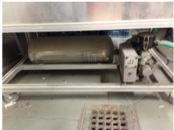
Figure 151a: The vacuum cleaner of the VaCo Mould & Figure 151b: The VaCo Mould in the future: equipped with a vacuum pump with a buffer tank
