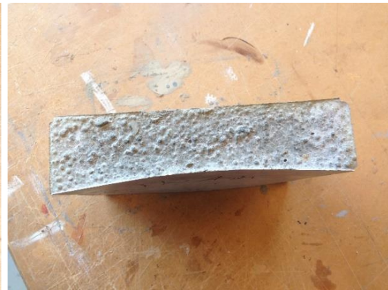
Figure 68a: Test fly ash as counter pressure material & Figure 68b: Result after demoulding
