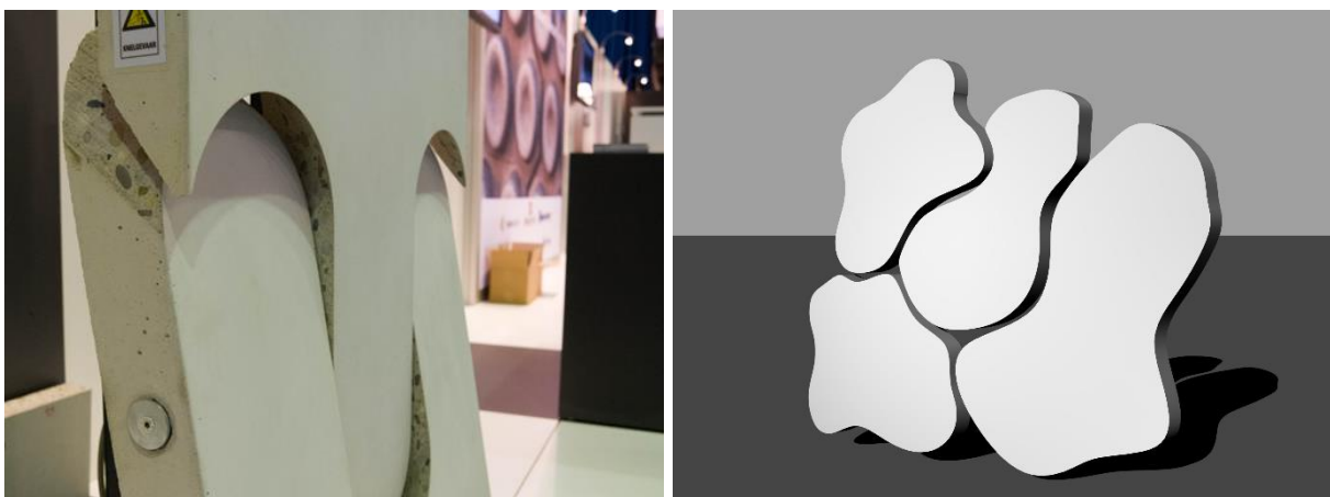
Figure 134a: Result of a six-axis water jet cutting machine (Bureaubakker, 2011) & Figure 134b: A render of concrete panels with organic/atlantic shapes
