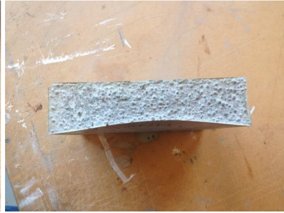
Figure 67a: Test sand as counter pressure material & Figure 67b: Result after demoulding
