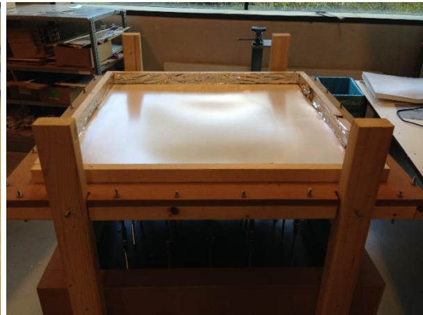
Figure 118a: Clamping the plastic sheet in the frame & Figure 118b: The frame is placed between the columns
