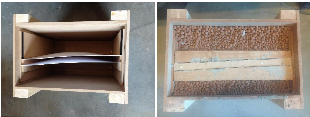
Figure 123a: The mould is placed in a box & Figure 123b: The mould is fully poured with concrete and clay granulate
