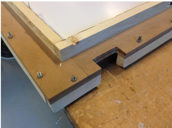
Figure 149a: Clamping the frame nowadays & Figure 149b: The VaCo Mould in the future: clamps to fixate the PS sheet
