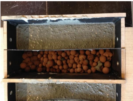
Figure 69a: Test clay granulate as counter pressure material & Figure 69b: Result after demoulding
