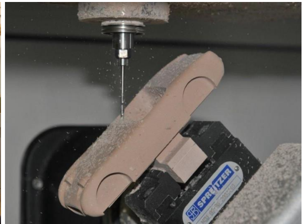
Figure 153a: The three axis milling machine of Eindhoven University of Technology & Figure 153b: A five axis milling machine (Vraagenaanbod.nl, 2011)
