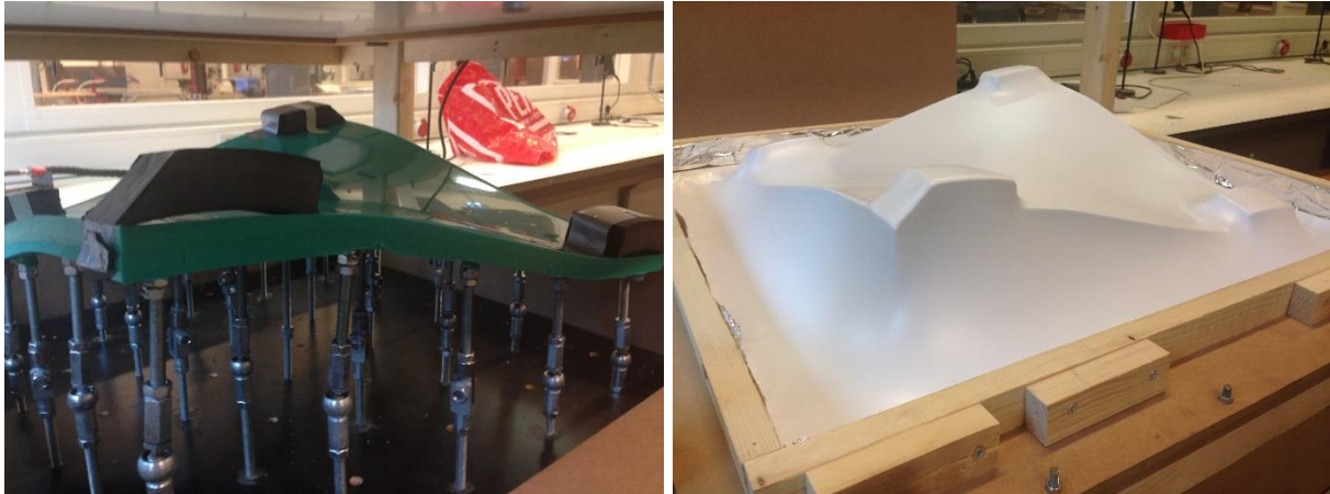
Figure 133a: Rubber on top of the flexible layer & Figure 133b: The result after vacuum forming with a local thickening
