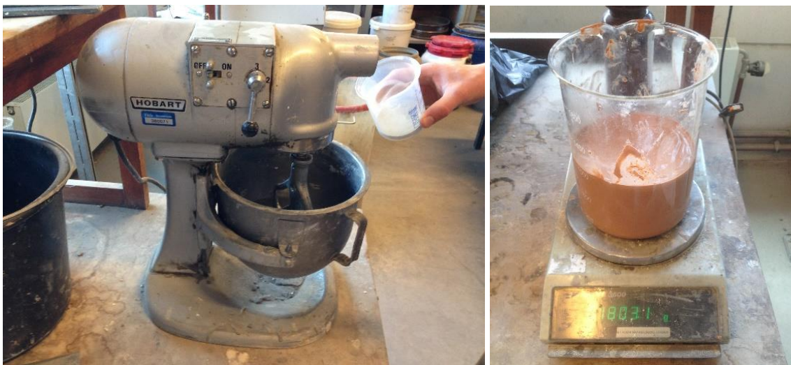
Figure 66a: The mixer that is used for the experiments (Hobart, Type N-50) & Figure 66b: The balance that is used for the experiments (Mettler PE3600)
