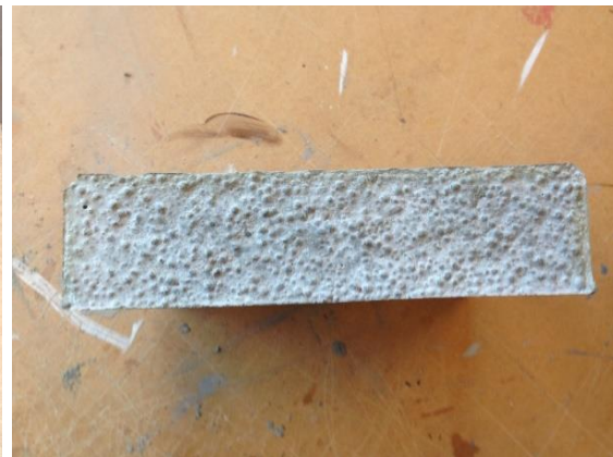
Figure 69a: Test clay granulate as counter pressure material & Figure 69b: Result after demoulding
