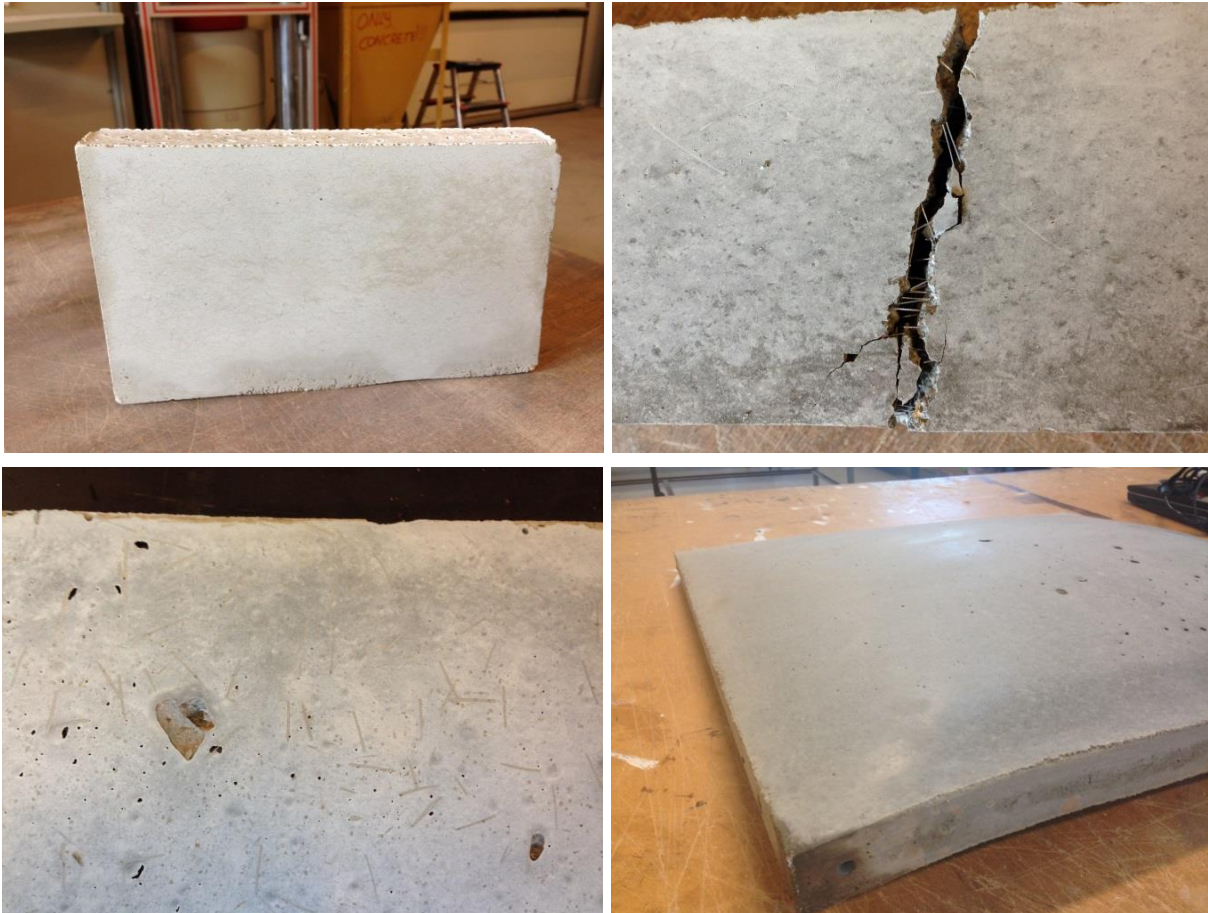
Figure 114a: Test panel, Figure 114b: The steel fibres sticks together, Figure 114c: The steel fibres are visible at the surface & Figure 114d: Result of testing the mixture on a large scale
