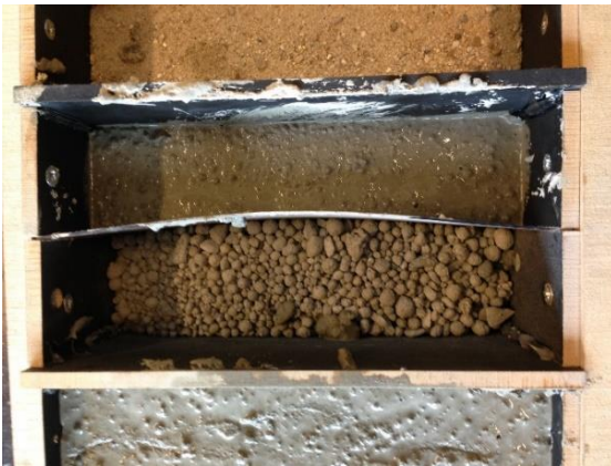
Figure 68a: Test fly ash as counter pressure material & Figure 68b: Result after demoulding
