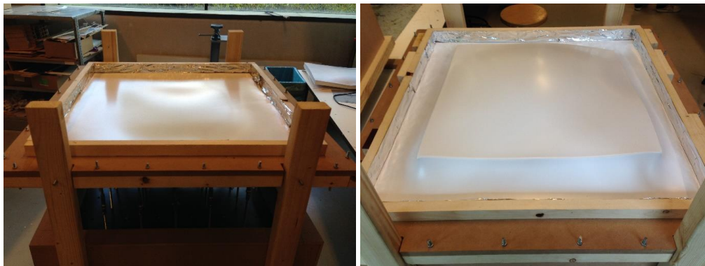
Figure 8a: The PS sheet is placed between the columns & Figure 8b: The PS sheet is pulled down over the flexible layer
