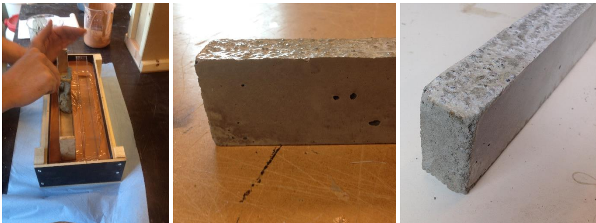
Figure 74a: Difficult to pour lightweight concrete in a small mould, Figure 74b: Result of pouring concrete in complete plastic mould & Figure 74c: Result of pouring concrete in wooden/plastic mould.
