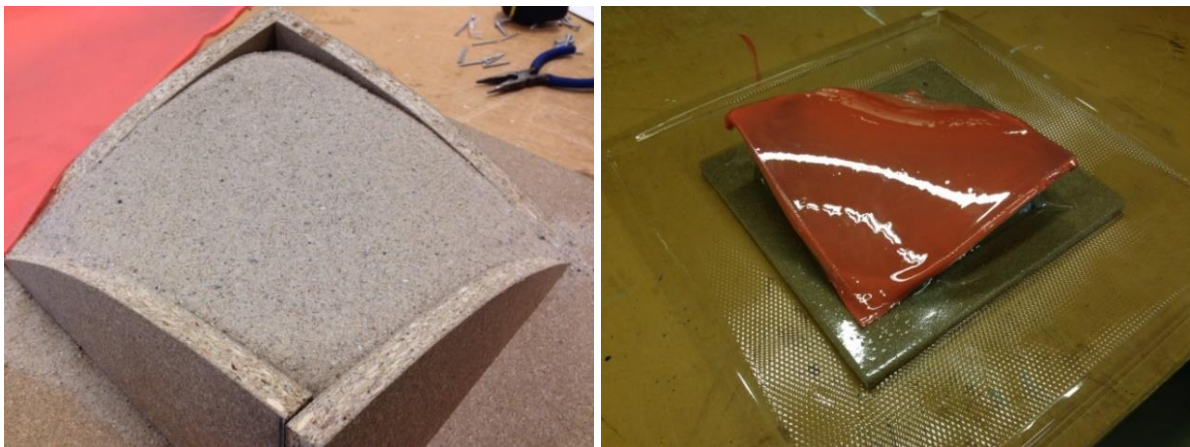
Figure 52a: Supported by sand & Figure 52b: No deformation
