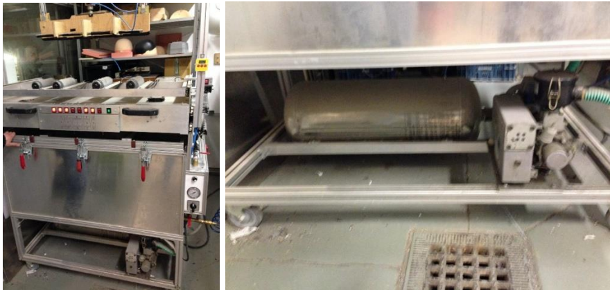
Figure 53a: Vacuum forming machine of Bas Hesselink IDAP & Figure 53b: Buffertank to control the pressure
