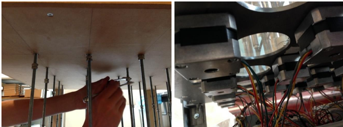
Figure 147a: The VaCo Mould nowadays & Figure 147b: The VaCo Mould in the future: controlled by a step motor
