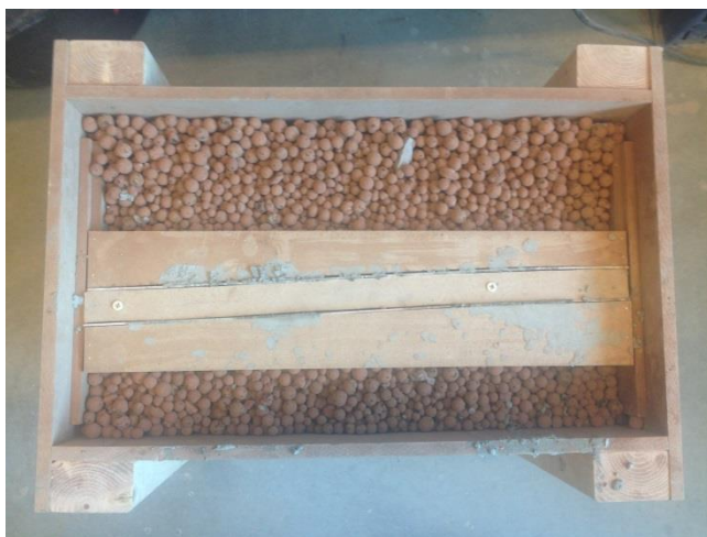
Figure 113a: Clay granules as counter pressure & Figure 113b: Clamping principle with milled wooden plates
