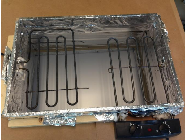
Figure 150a: The heating element of the VaCo Mould & Figure 150b: The VaCo Mould in the future: a heating element with heating spirals
