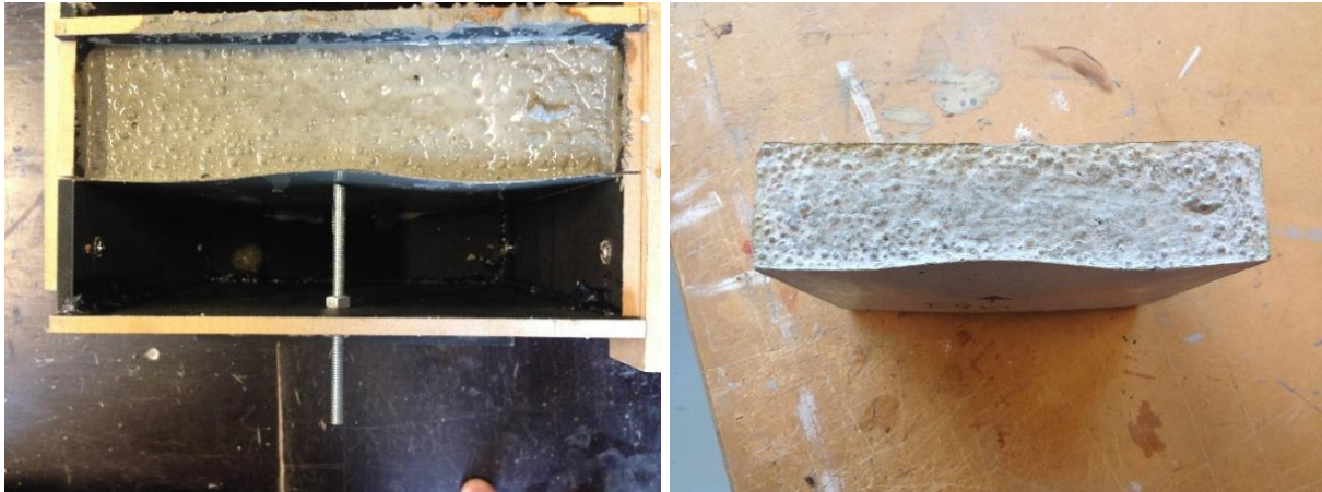
Figure 70a: Test pin as counter pressure & Figure 70b: Result after demoulding
