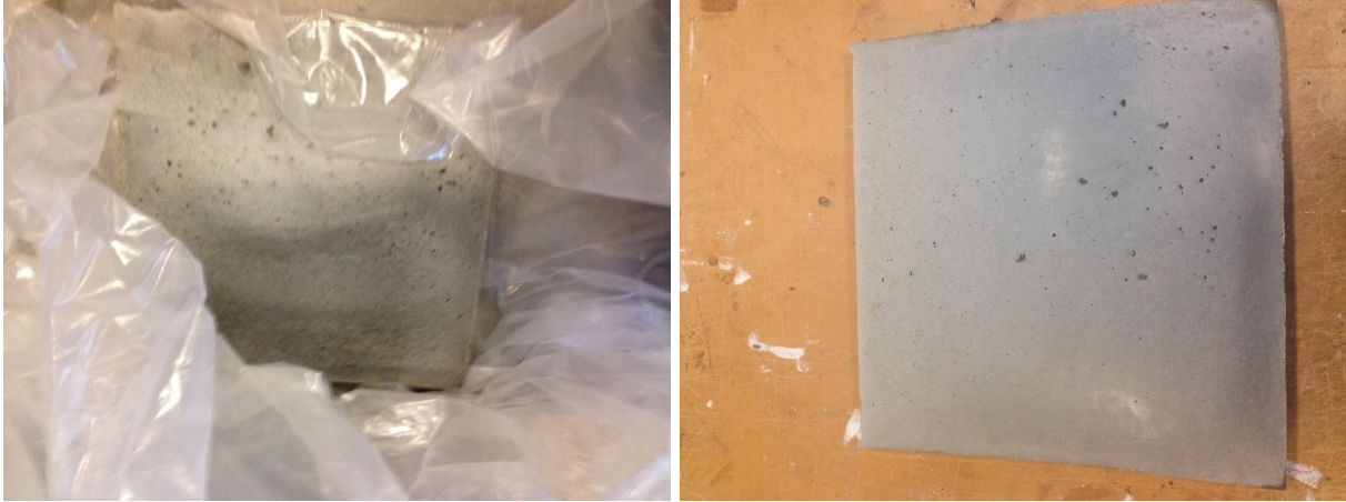
Figure 124a: A concrete panel wrapped in shrink foil & Figure 124b: The concrete panel cured after four days
