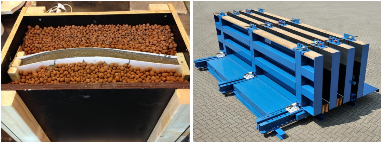
Figure 154a: The pouring process of the VaCo Mould & Figure 154b: A battery mould for prefabricated houses (Hendriks Precon, 2015)
