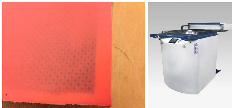
Figure 50a: Spring steel mesh in a silicon layer & Figure 50b: The Formech 686 vacuum forming machine (Scouten Group, 2015)
