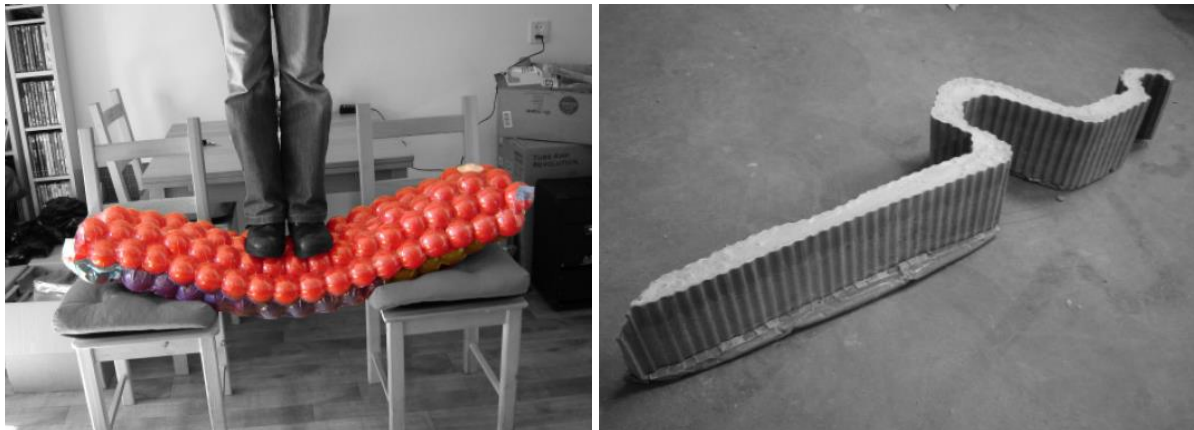
Figure 28a: The principle of Vacuumatics & Figure 28b: A concrete element that is made with the technique of Vacuumatics (Huijben, n.d.)
