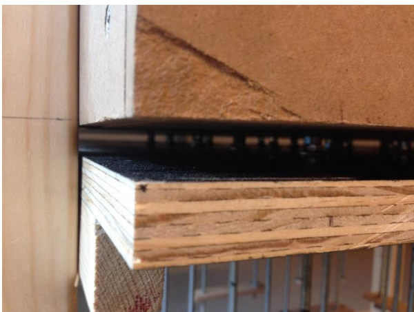
Figure 117a: No clearance between the nuts and the airtight box, Figure 117b: The flexible layer is set in a double curved form
