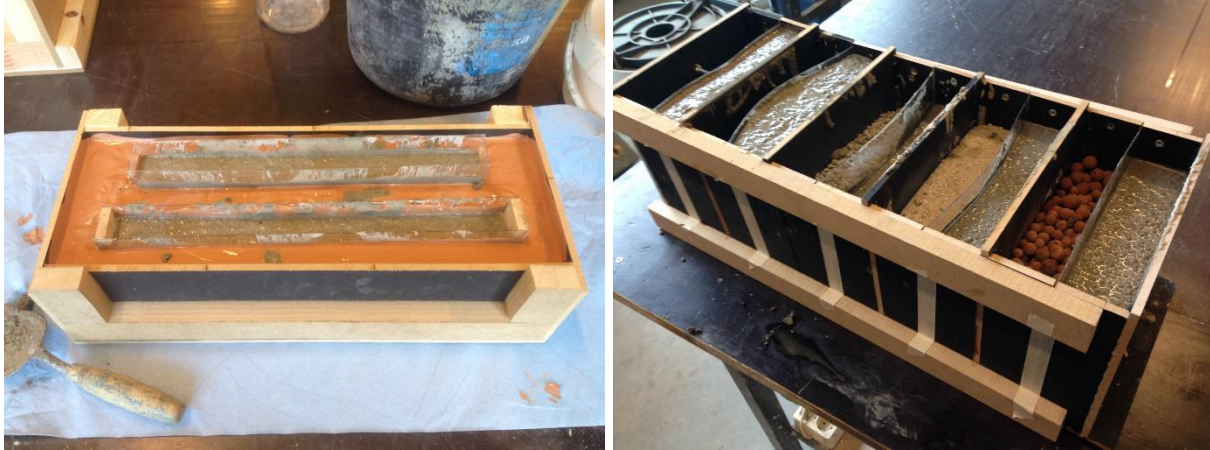
Figure 63a: Counter pressure for lowering process & Figure 63b: Counter pressure for fixating process
