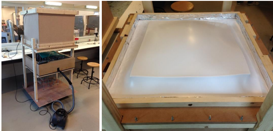
Figure 120a: Mould setup before vacuum forming & Figure 120b: The PS sheet is pulled down over the flexible layer
