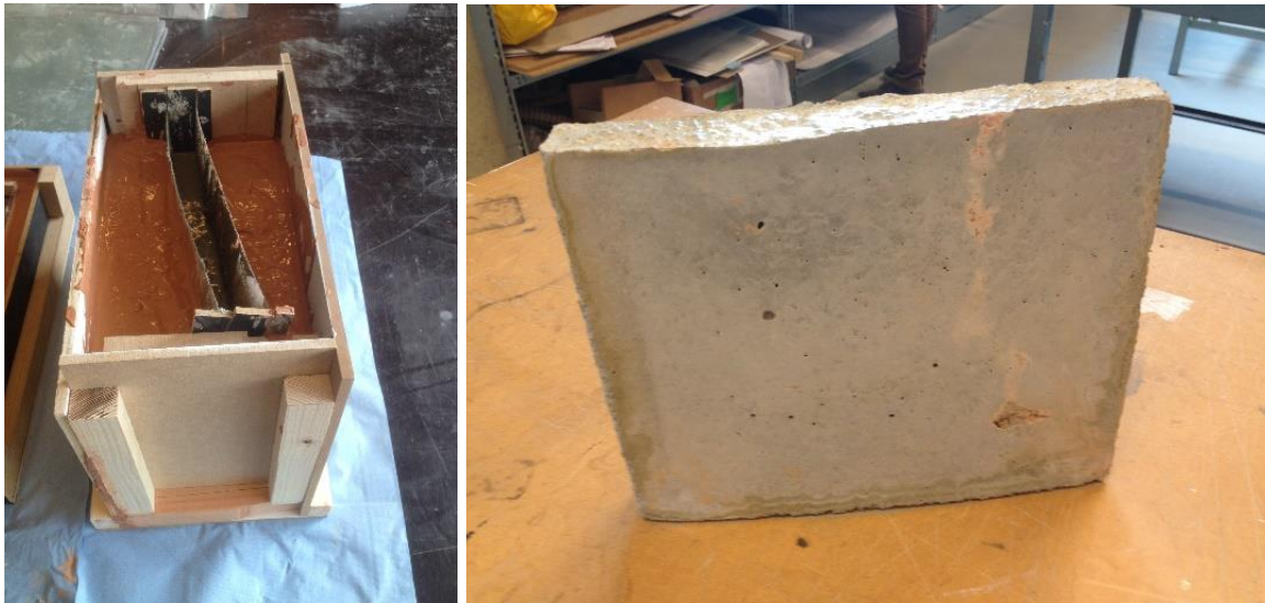
Figure 76a: Clamped plastic sheets in a basin & Figure 76b: The result of casting a double curved concrete element with lightweight concrete
