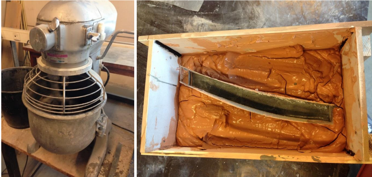
Figure 77a: Hobart (Type A-200) mixer & Figure 77b: Lowering process in the bentonite
