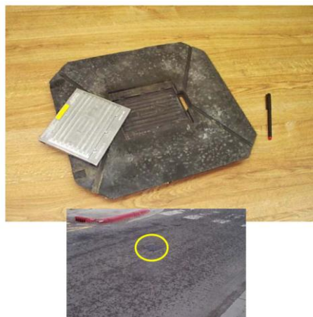
Figure 3-4 Magnetic detector NuMetrics NC-97 (Mcgowen & Sanderson, 2011)
