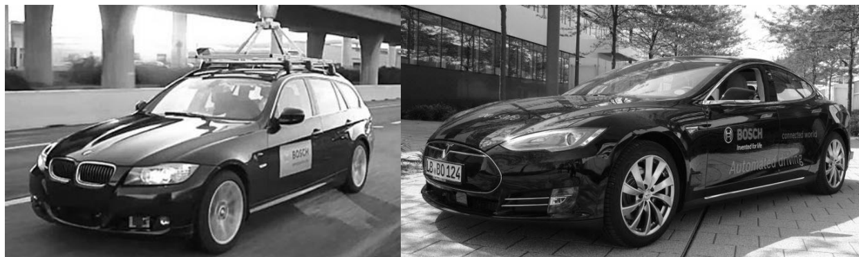
Figure 15: BMW 325D (left) and Tesla Model S (right) autonomous prototypes of Bosch
