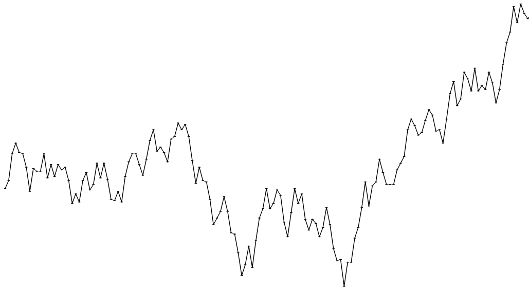
Figure B.3: Semi-random generated data set with 150 cells and elevations in between 0 and 211, the dispersion was set to 20.
