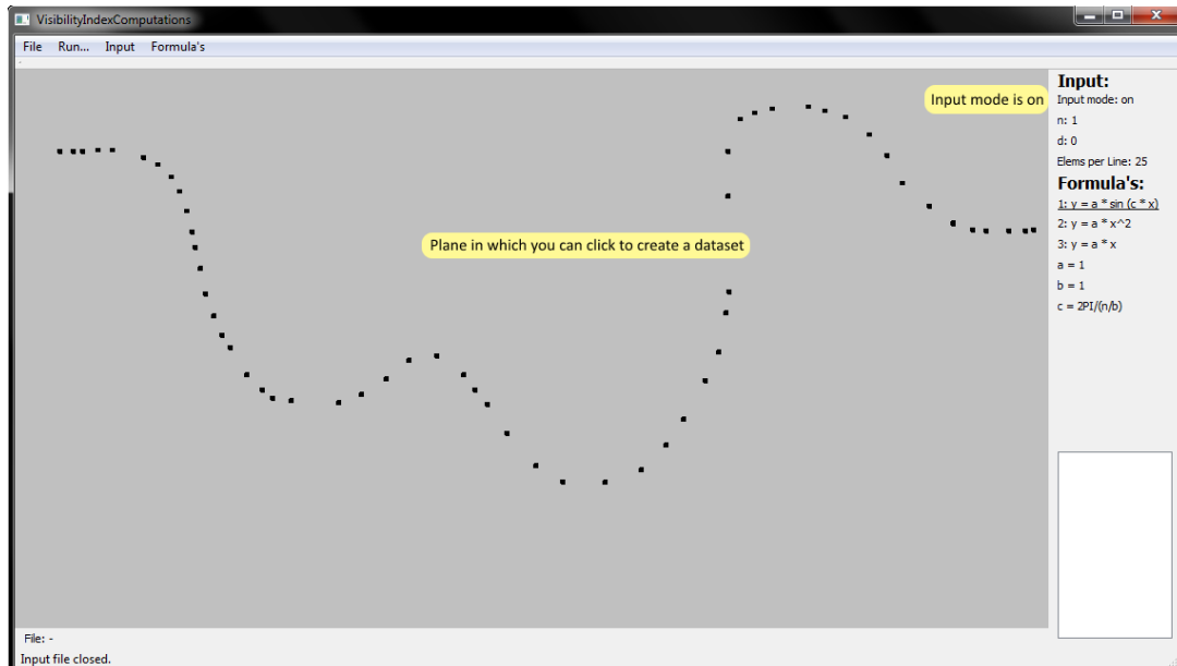
Figure 5.2: An annotated screenshot of the GUI when in input mode.
