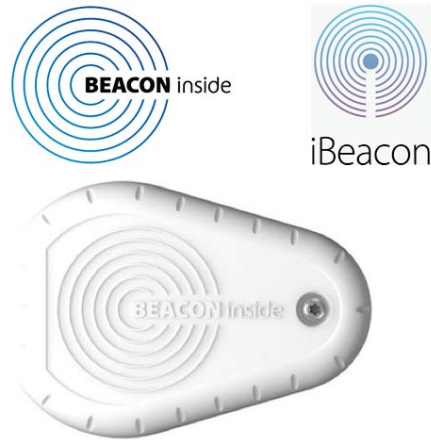
Figure 4.4: BEACONinside node, a clone of iBeacon.
