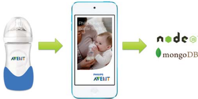
Figure 6.1: The communication scheme from uBottle to the server
