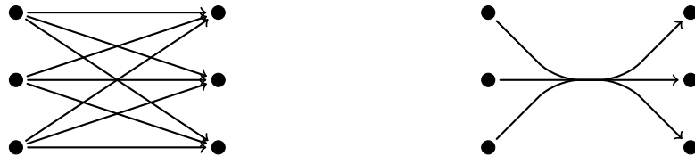
Figure 2.1: The idea of confluent drawings: we represent every edge from the original directed complete bipartite graph K_{3,3} (left) by a smooth curve in the confluent drawing (right).
