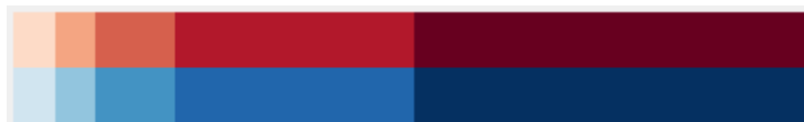
Figure 5.4: In a discrete colormap, the range boundaries can be shifted obtain a more effective color distribution.
