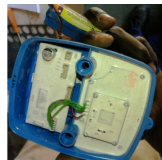
Figure 4: Opened up prepaid water meter with the electronics and battery unit.
