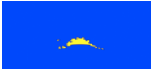
Figure 5.2.3: Less detail in side lobes due to reduced dimensions in depth buffer.
