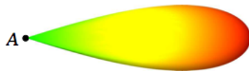
Figure 3.3.4: Top view of a collection of antenna patches in the shape of the radiation pattern; patches with a warmer color give off more light. [3]
