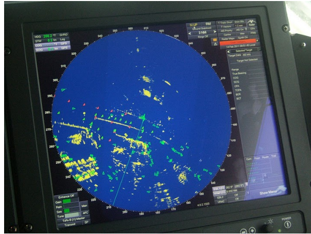
Figure 1.0.1: A modern radar system showing part of the Nieuwe Waterweg.
