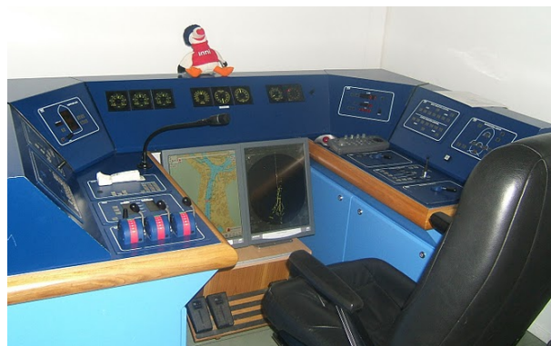
Figure 1.0.2: A radar training station at the Scheepsvaart Transport College in Rotterdam. The radar simulation is visible on the center-right monitor.
