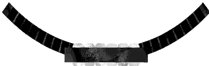
Figure 5.17: The initial mover on a circular curved backplate with a diameter of 0.9m , top view.
