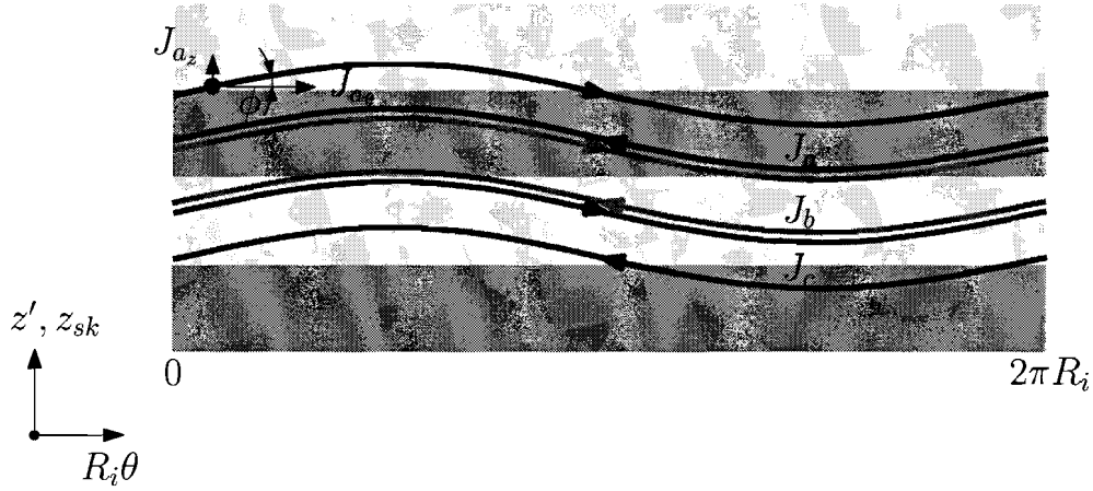
Fig. 4.5: Schematic view of sinusoidal stator skewing.
