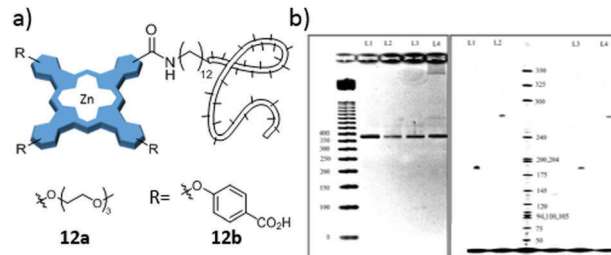
Fig. 20 (a) Scheme of Zn(II)Pc derivatives 12a and 12b as labelling agents in oligonucleotide PCR. (b) Images of agarose (left) and polyacrylamide (right) gels after electrophoresis of PCR products. Detection was accomplished using UV absorption at 254 nm after staining the gel with ethidium bromide (left) or near-IR fluorescence at 700 nm (right). Adapted with permission from ref. 191. Copyright 2007 American Chemical Society.
