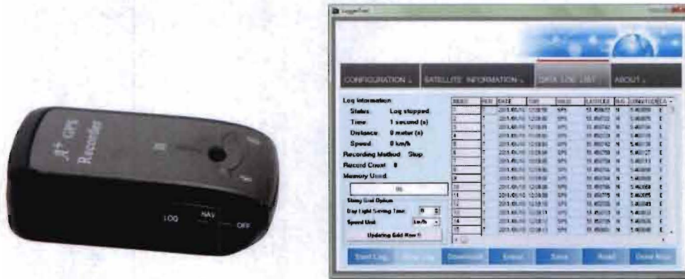
Figure 3.6 The GPS-tracker participants carried with them during the experiment. Left: GPS trip recorder, model 747 A+. Right: the interface on the PC for reading the data from the tracker.
