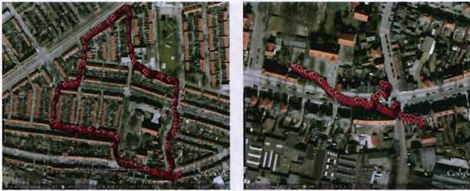
Figure 4.4 Examples of the visualisation of tracker data in Google Earth. Left: the route is complete but the data sometimes show the participant walking through houses. Right: messy and incomplete data.
