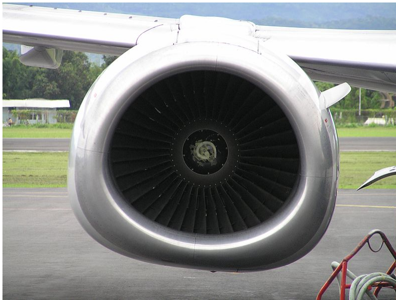
Figure 1.1: Non-circular duct profile of the CFM56 engine in a Boeing 737-500: Hamster Pouch
