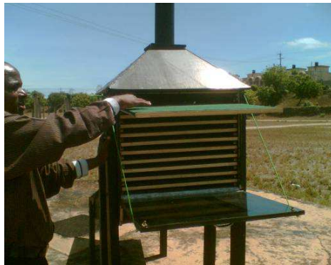
Figure 3.14: The trays that are used in the design by TIRDO are not suitable according to CAC standards
