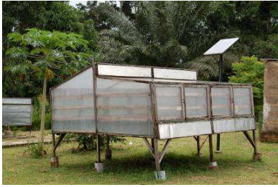
Figure 3.7: UDSM Solar Dryer with forced air circulation
