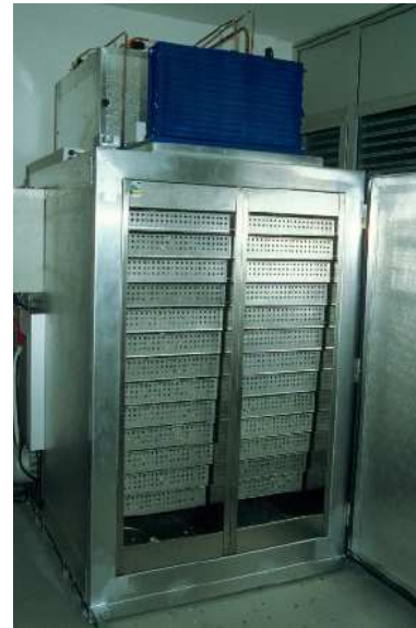
Figure 3.15: A Cabinet dryer as produced in Germany by Innotech Ingenieursgesellschaft mbH
