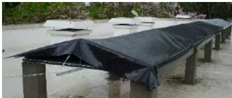
Figure 3.17: Application of foil for light sensitive products
