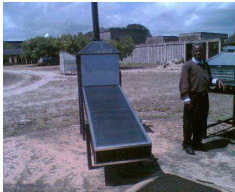
Figure 3.13: A small scale cabinet dryer produced by TIRDO in Tanzania. The dryer uses airflow by natural convection
