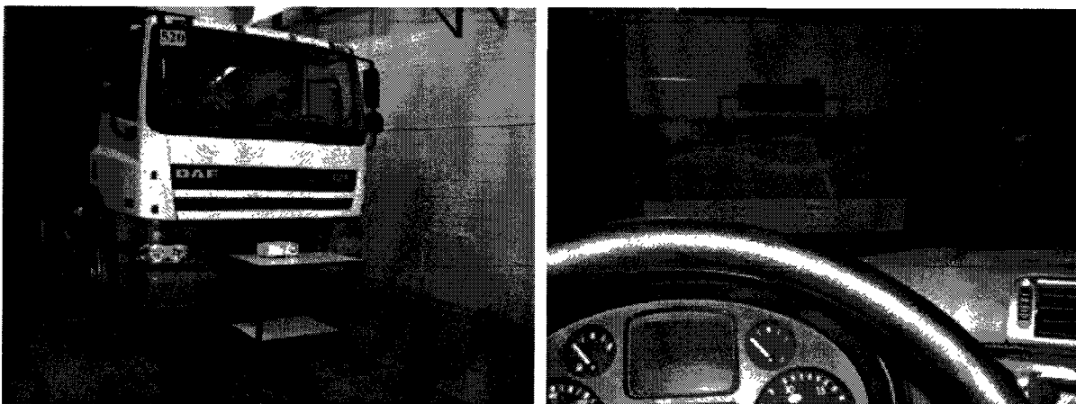
Figure 6. At the left panel: experimental setup with truck and beamer; at the right panel: view from the driver's position showing the screen on which the traffic situations and questionnaires are presented.
