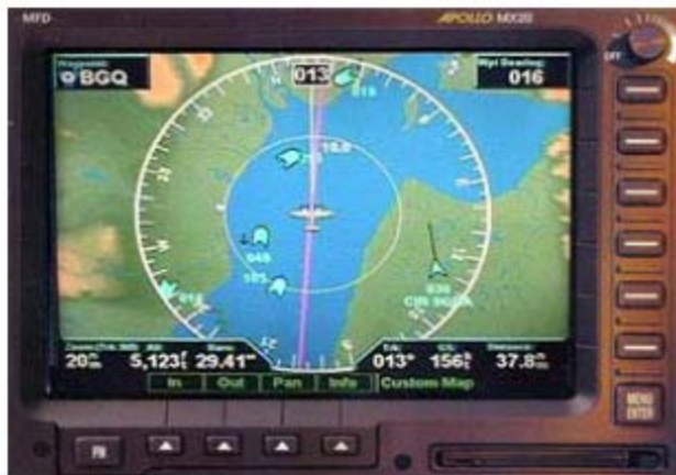
Figure 3. In this display, traffic can be seen superimposed on the surrounding terrain. The information is received live from other transmitting aircraft and from the ground-based transceiver.
