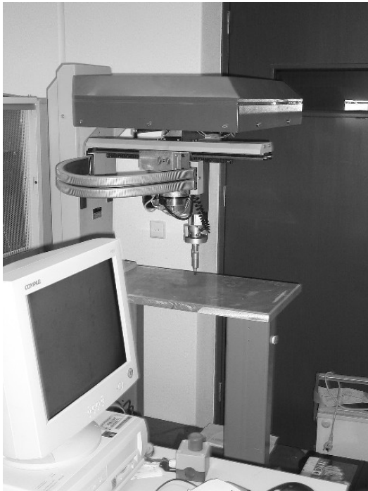
(a) Robotic system consisting of two independent driven axes.
