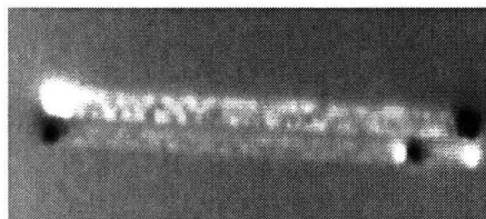
Figure 4.34: MFM scan of two strips. The scan size is 23 \times 10 \mu\text{m} . The top strip has a width of 1.5 \mu\text{m} , and the bottom strip is 1.0 \mu\text{m} wide. The magnetization of both strips is opposite, although the field history is not known. It is clear that the ends of the strips show magnetic contrast, but also an internal structure is visible. The bottom strip clearly shows a domain wall.
