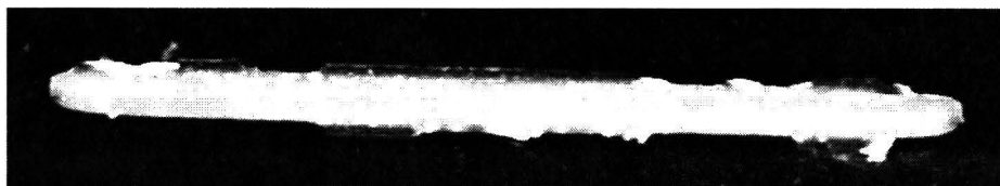
Figure 4.31: AFM image of a CoFe strip with length 20\ \mu\text{m} , and width 1\ \mu\text{m} . The edges of the strip are rough due to the sample preparation. The image is 22 \times 4\ \mu\text{m} .
