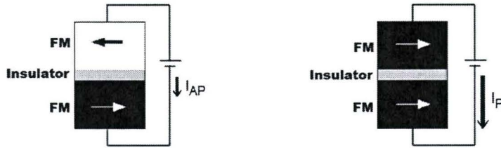
Figure 1.3: Schematic overview of a magnetic tunnel junction (MTJ). A thin insulator is sandwiched between two ferromagnetic (FM) layers which are connected to two electrodes. The arrows in the (FM) layers indicate the magnetization direction. The tunnel current of a MTJ-device is dependent on the orientation of the magnetization. When applying a bias voltage across the structure, an anti-parallel orientation (left) leads to a high resistive state, and thus a low current ( I_{AP} ) while a parallel orientation (right) results in a low resistance, and high current ( I_P ).
