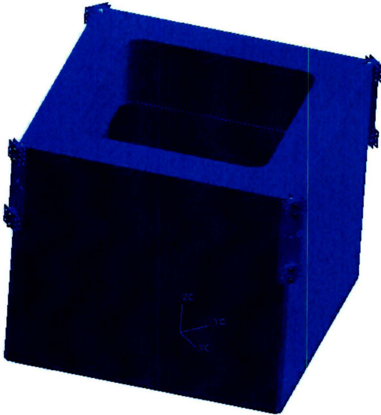
Figure 8.3.5: Main frame with connection points for the suspension rods at the corners
