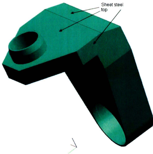
Figure 8.1.9: Wheel carrying arm: steel tube with two pieces sheet steel, angle iron, two partitions, lower sheet steel above the tire, machined cylinder, a partition for support of the cylinder and the top steel sheet.
