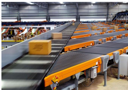
Figure 29 Infeed zone, the infeeds (right) place the packages on the sorter (left)
