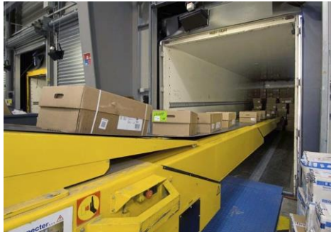
Figure 28 Extendable to ease unloading/loading trucks
