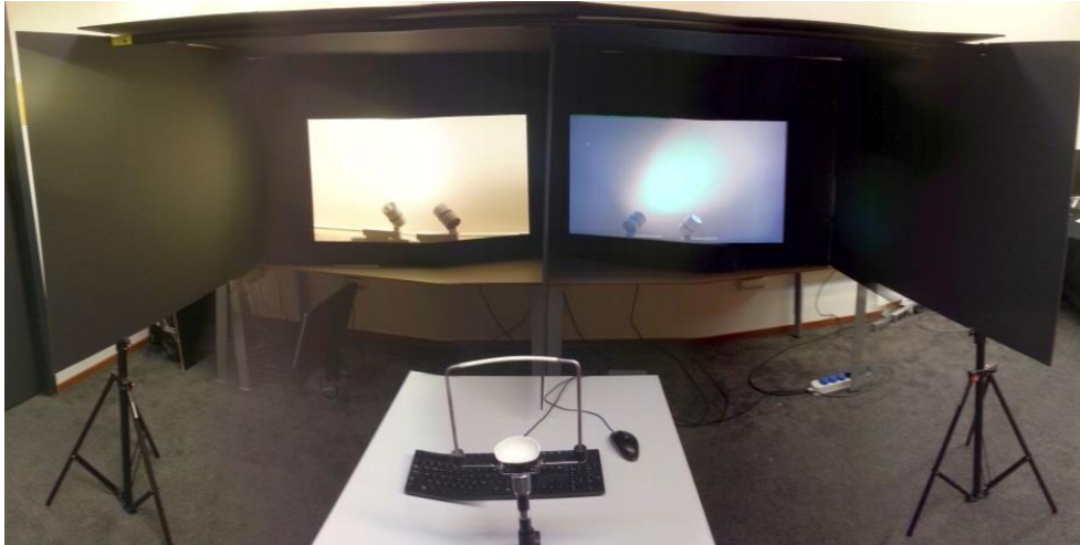
Figure 9: Panorama photograph of the viewing box; on the left the real-world scene; on the right the display showing the virtual scene
