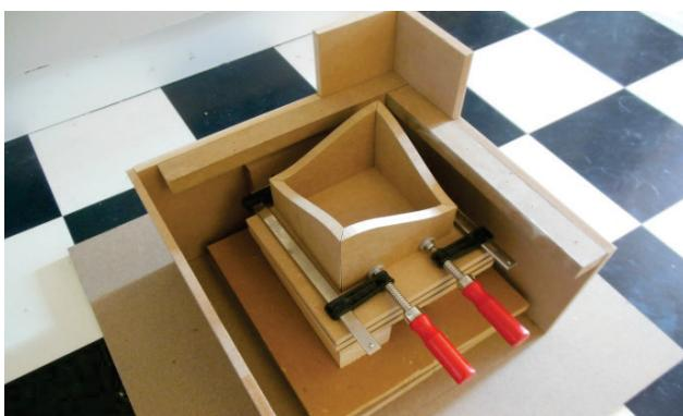
Figure 3.19: Static edge mould method setup
