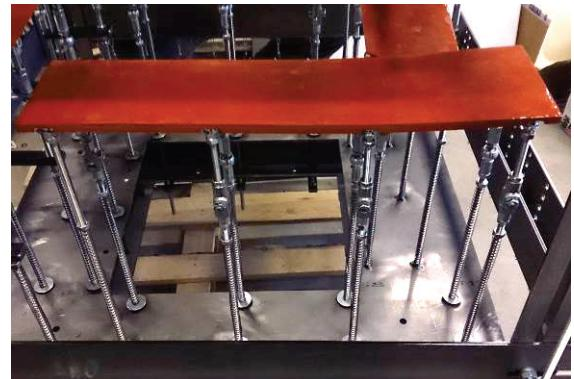
Figure 4.43: Flexible edge of silicone rubber jointed to the pendulum rods
