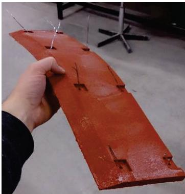
Figure 4.42: Result of the silicone rubber reinforced with a spring steel mesh
