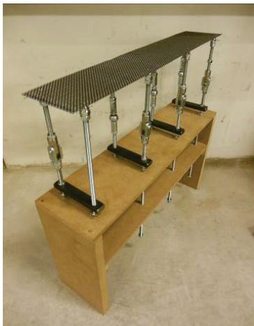
Figure 4.38: Side view of spring steel mesh in flat position
