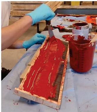
Figure 4.41: Casting the silicone rubber into the wooden mould. The spring steel mesh is attached to the mould
