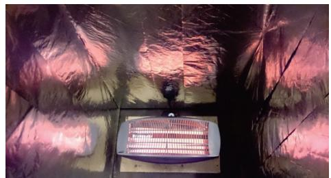
Figure 4.27: Uniform heat distribution due to reflection of radiation
