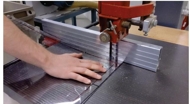
Figure 7.17: Cutting the thermoplastic to size with the use of a band saw
