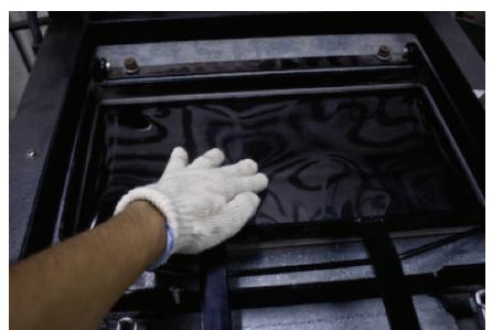
Figure 4.30: After a period of time, the red heat panel can be pulled back and the thermoplastic is ready to be deformed. (adapted from National University of Singapore)
