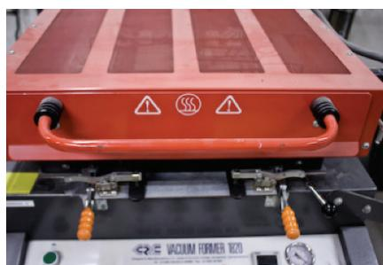
Figure 4.29: Once the sheet is secured, the movable red heat panel can be pulled out (adapted from National University of Singapore)
