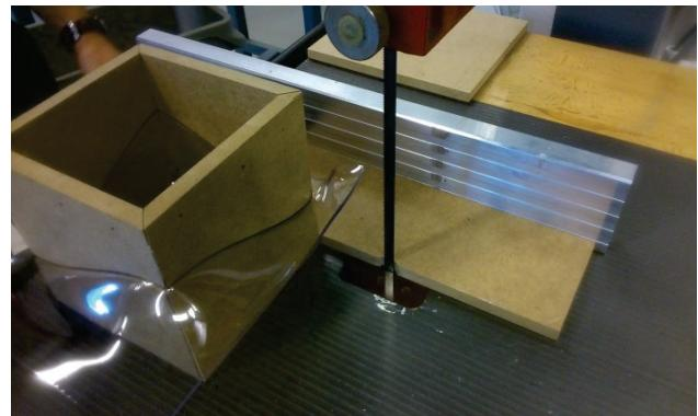
Figure 3.22: Sawing thermoplastic sheet of 250x250x3mm to a sheet of 150x150x3mm
