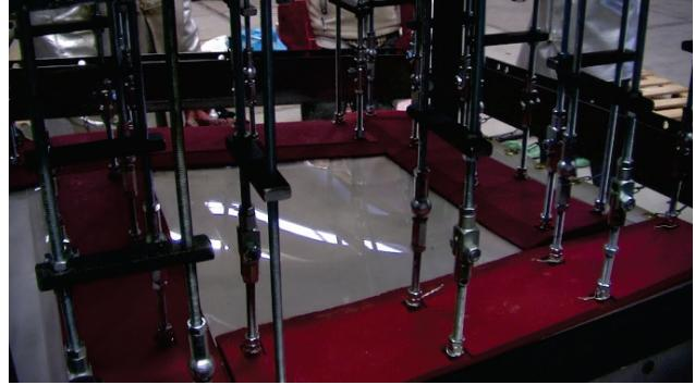
Figure 7.15: Drawing contours flexible edges and let the thermoplastic sheet cool
