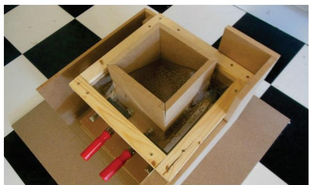
Figure 3.20: Heated thermoplastic sheet between static edge moulds
