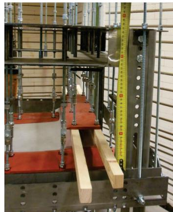
Figure 7.3: Fixating the side rod to obtain a zero level
