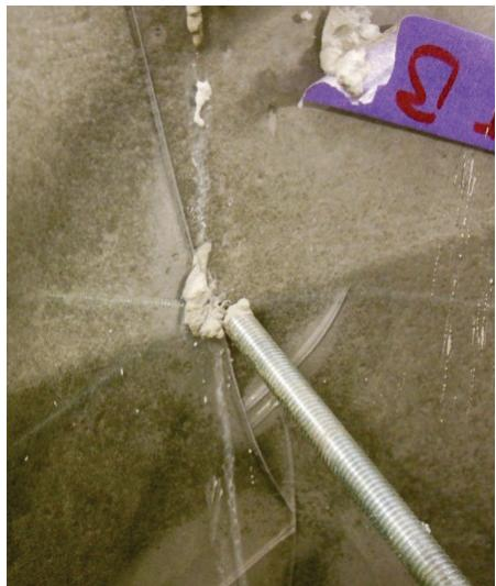
Figure 7.22: Cracks in thermoplastic sheet
