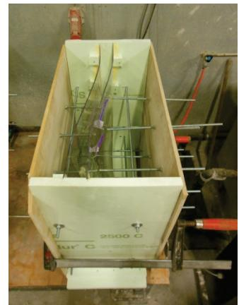
Figure 7.20: Formwork supported with pins
