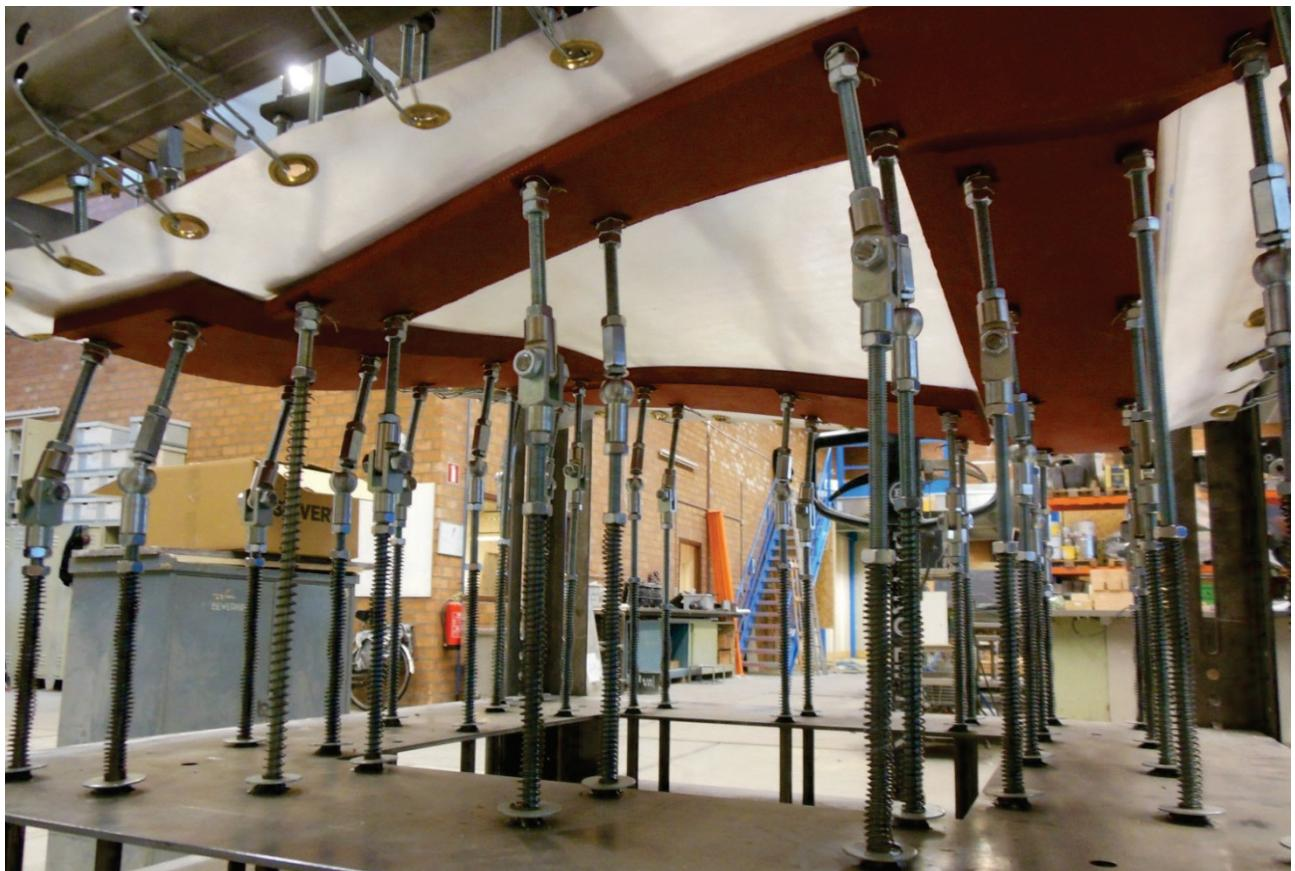
Figure 4.52: Lower actuators of the Fluid Mould
