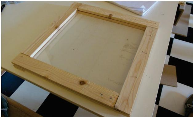
Figure 3.17: Thermoplastic sheet of 250x250x3mm clamped in wooden slats
