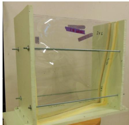
Figure 7.19: Seal formwork seams
