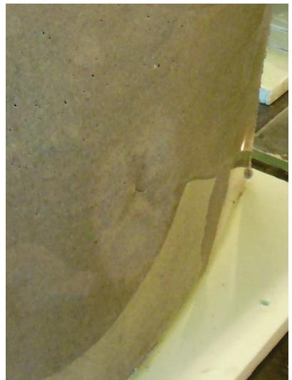
Figure 7.23: Crack thermoplastic visible at concrete surface
