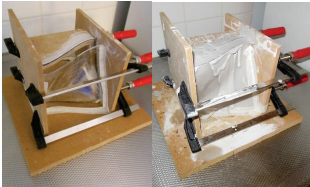
Figure 3.23: A closed mould is created through clamping two sheets between wooden boards.
