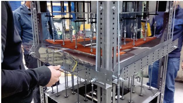
Figure 7.16: Removing the deformed thermoplastic sheet
