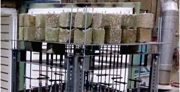
Figure 7.6: Lifting plate supported by the distance holders
