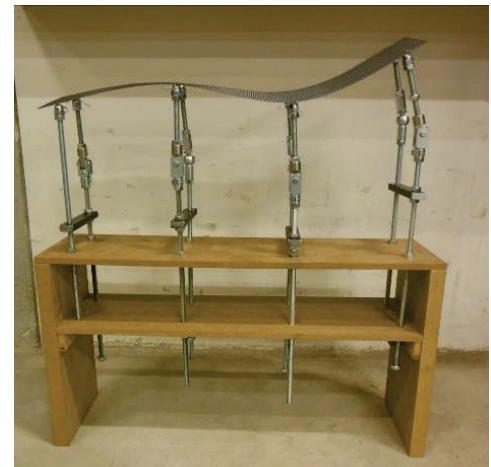
Figure 4.40: Front view of spring steel mesh in curved position
