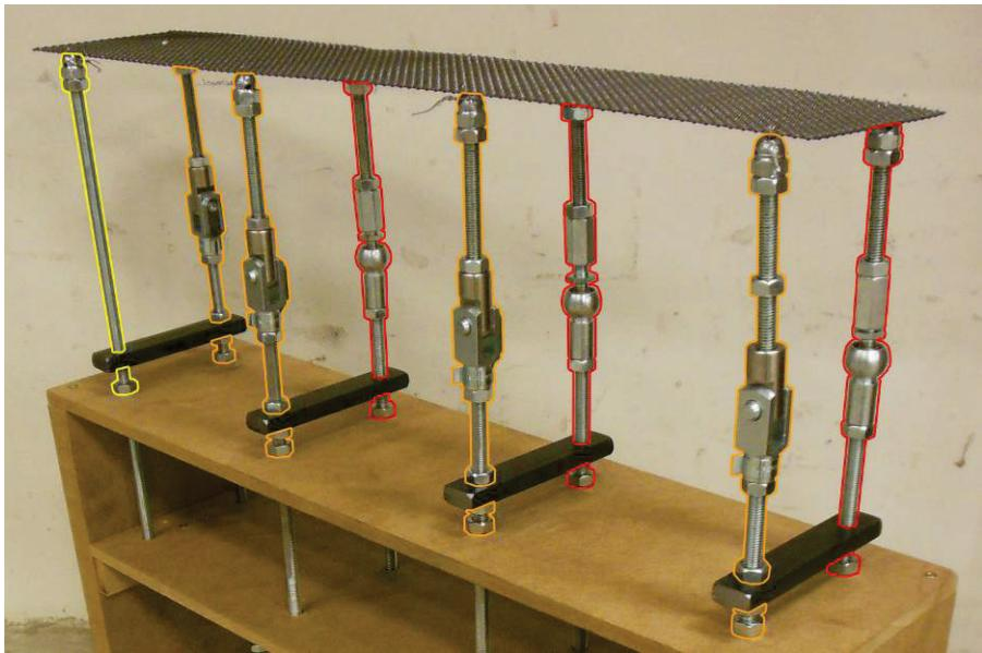
Figure 4.35: Setup of the pendulum rods. The yellow rod is a non-pendulum rod, the orange rods are clevis eye connections and the red rods are ball joint connections
