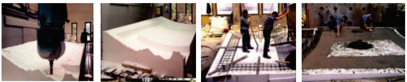
Figure 1.5: CNC milling Styrofoam moulds for the casting of reinforced concrete panels for The New Zollhof by Frank O. Gehry (adapted from Kolarevic)
