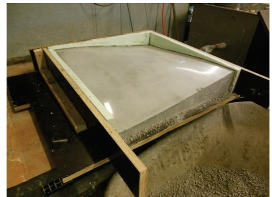
Figure 7.30: Formwork after removing the granules
