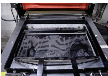
Figure 4.28: A thermoplastic sheet is secured to a vacuum former by pressing down a lever (adapted from National University of Singapore)
