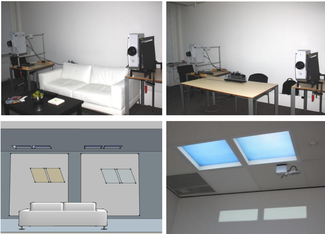
Figure 16: Top left figure shows photograph of home setup. Top right figure shows photograph of office setup. Bottom left figure shows graphical representation of setup. Bottom right figure shows photograph of projected (small rectangular) sun pattern.
